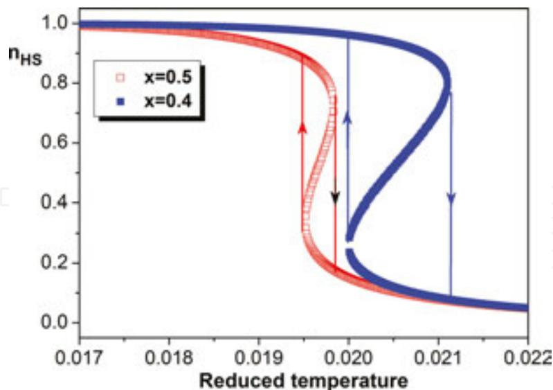
**Figure 15.** Static LITH for two values of the interaction parameter  $x$ . Parameters used in these calculations are  $y = 0$ ,  $\delta_0 = 0.6$ ,  $x = 0.1$ ,  $\ln g = 5$ ,  $N = 2000$ ,  $A = 0.8$ ,  $k_\infty = 100$ ,  $I_0 \sigma_a = 5 \times 10^{-4} \text{ s}^{-1}$ .
