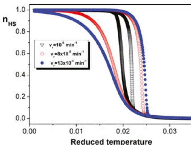
**Figure 16.** Dynamics LITH for three values of the temperature change rate  $v_r$ . Parameters used in the calculations are  $x = 0.5$ ,  $y = 0$ ,  $\delta_0 = 0.6$ ,  $\alpha = 0.1$ ,  $\ln g = 5$ ,  $N = 2000$ ,  $A = 0.8$ ,  $k_{\infty} = 100$ ,  $I_0\sigma_a = 5 \times 10^{-4} \text{ s}^{-1}$ .
