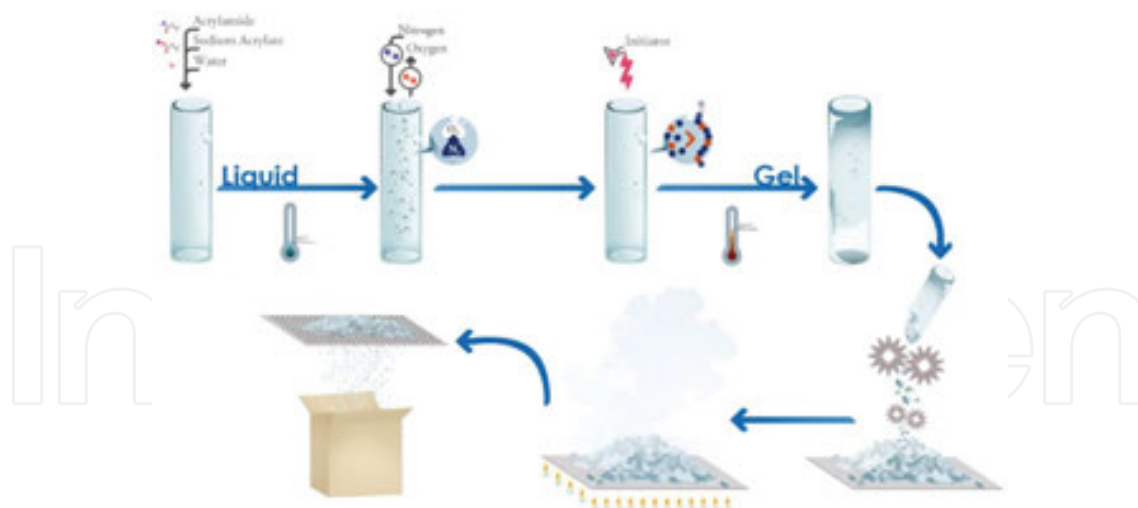
Figure 7. Overview of the copolymerization process [25].
