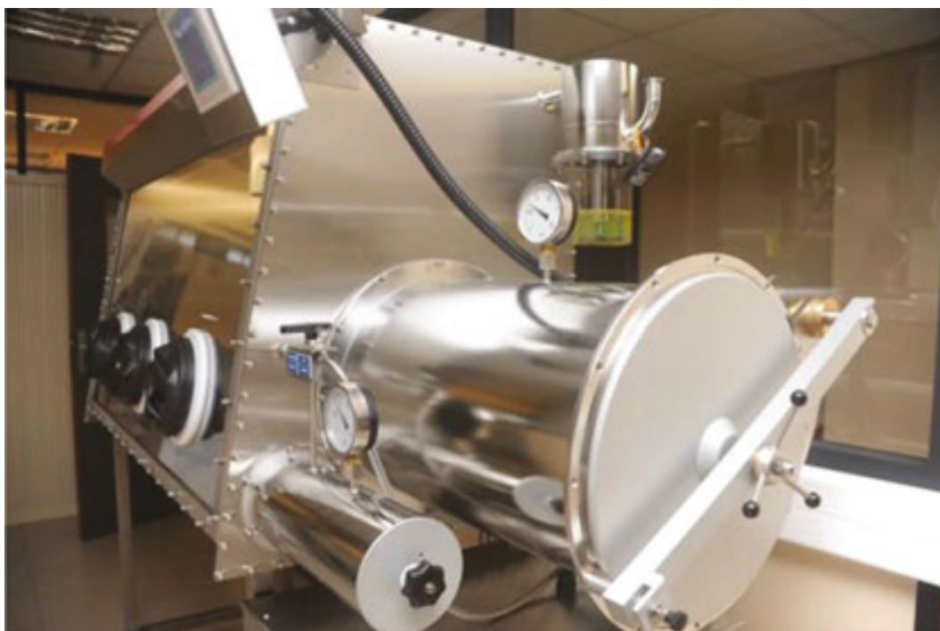
Figure 15. Typical glove box set-up to perform tests in anaerobic conditions [25].
