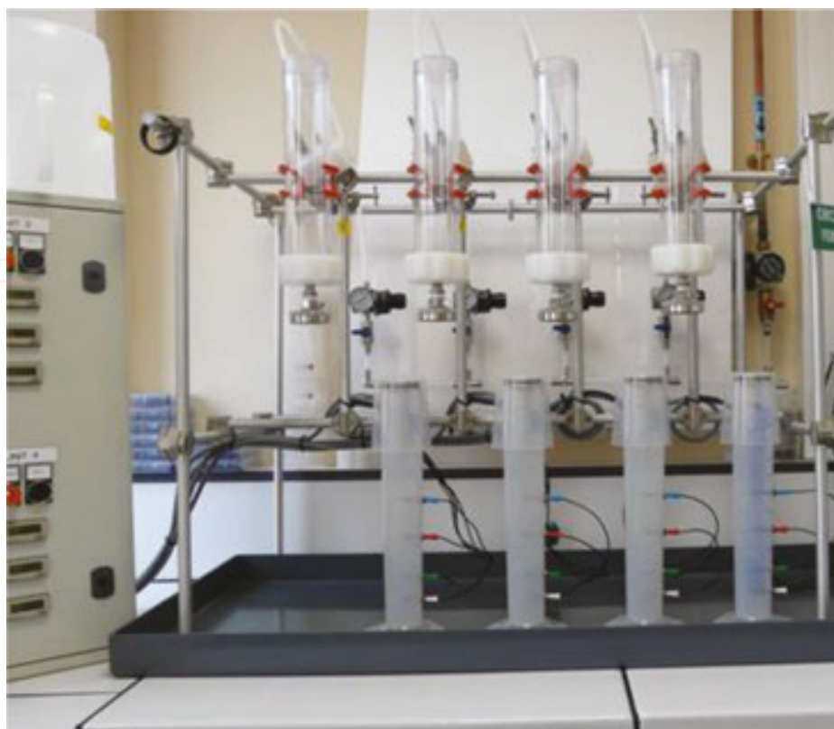
Figure 23. Typical set-up used to perform filter ratio tests with vessels (top) and graduated cylinders connected to a stopwatch (bottom) [25].
