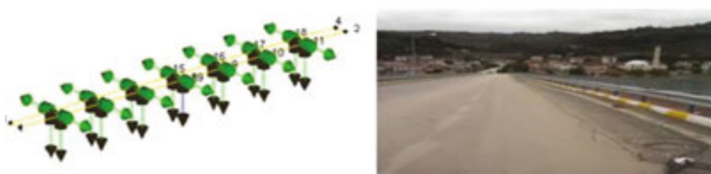
Figure 18. Accelerometer location and views taken from the measurements.
