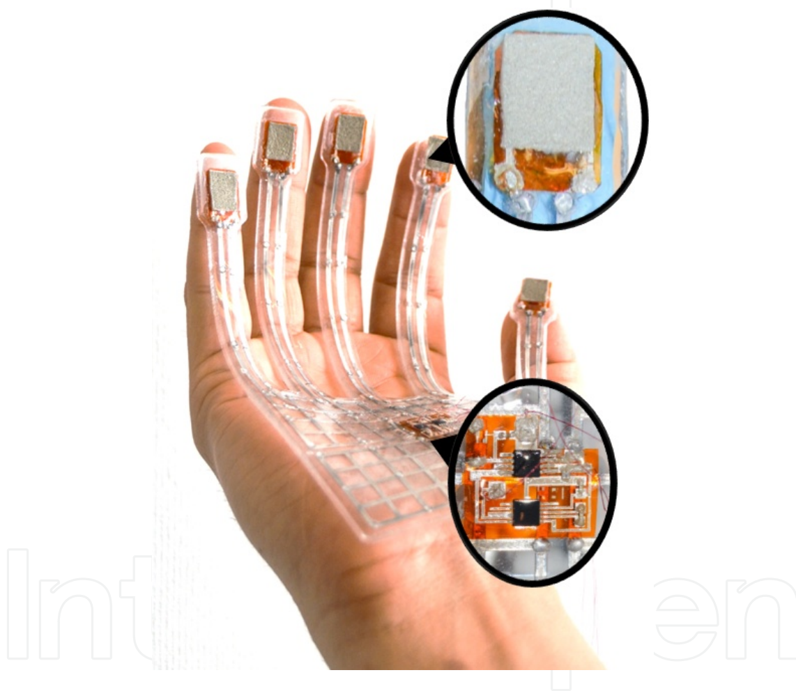
Figure 28. Photograph of the stretchable multi-point, wireless pressure sensor prototype.
