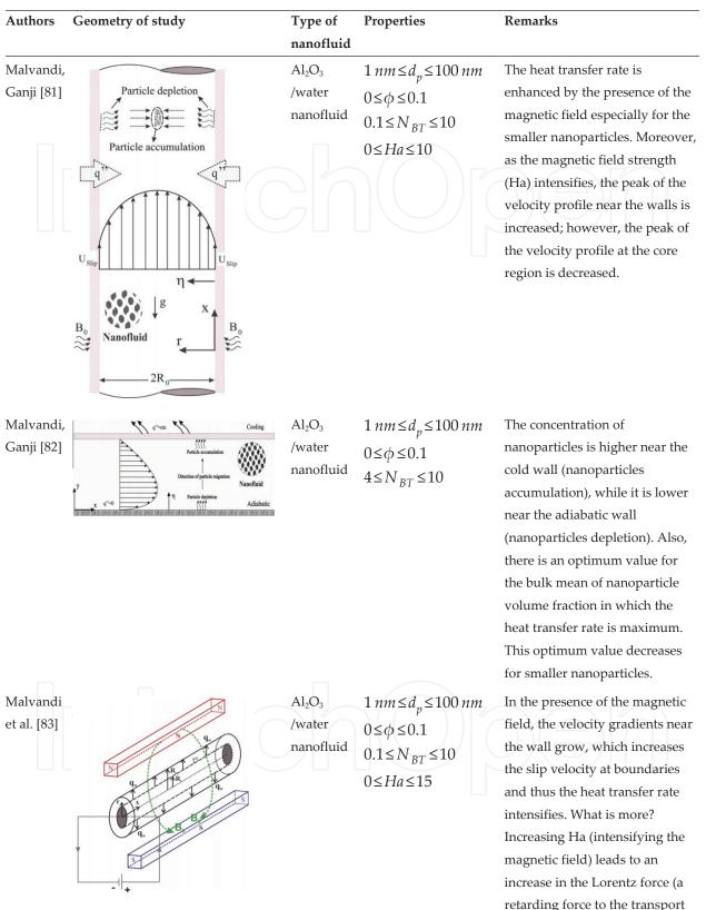
magnetic field) leads to an increase in the Lorentz force (a retarding force to the transport phenomena), which tends to resist the fluid flow and thus reduces the flow's velocity.
