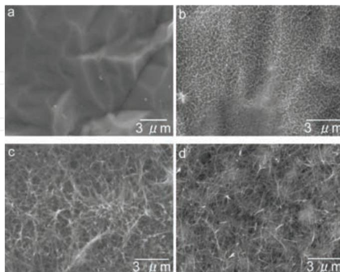
**Figure 10.** SEM images of sodium titanate nanofiber thin films synthesized following different reaction times; the titanium plate before the synthesis (a), and after 1 h (b), 5 h (c), and 12 h (d) reaction times [10].
