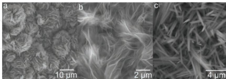
**Figure 7.** SEM images of the hexagonal  $\text{Ti}(\text{HPO}_4)_2\cdot\text{H}_2\text{O}$  nanoplate thin film (a), the  $\text{Ti}_2\text{O}_3(\text{H}_2\text{PO}_4)_2\cdot 2\text{H}_2\text{O}$  nanosheet thin film (b), and the  $\text{Ti}_2\text{O}(\text{PO}_4)_2\cdot\text{H}_2\text{O}$  nanorod thin film (c).
