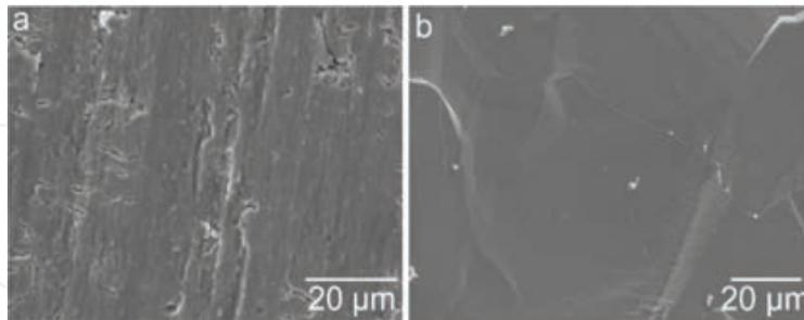
**Figure 1.** SEM images of the titanium plates before (a) and after (b) the HF treatment.
