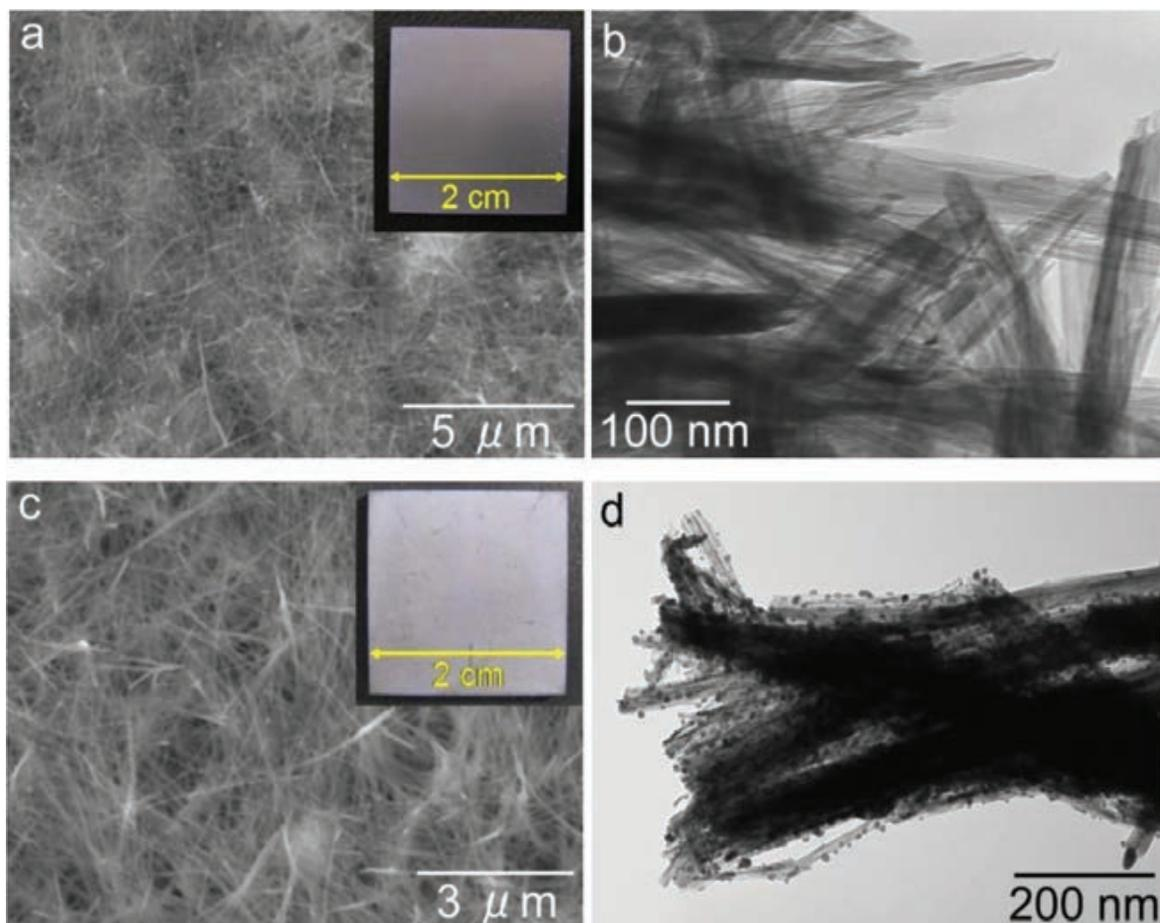
**Figure 8.** SEM images (a and c) and TEM images (b and d) of the sodium titanate nanofiber thin film (a and b) and the silver nanoparticles/silver titanate nanofiber thin film (c and d). Insets are photographs taken with a digital camera [10].
