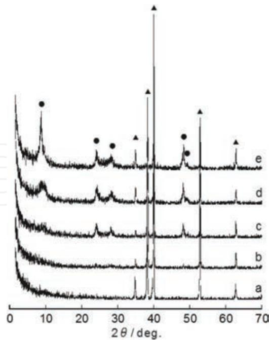
**Figure 11.** XRD patterns of sodium titanate nanofiber thin films following different reaction times; the titanium plate before the synthesis (a), and after 1 h (b), 5 h (c), 12 h (d), and 20 h (e) reaction times. Peak assignment: ●, sodium titanate; ▲, titanium [10].
