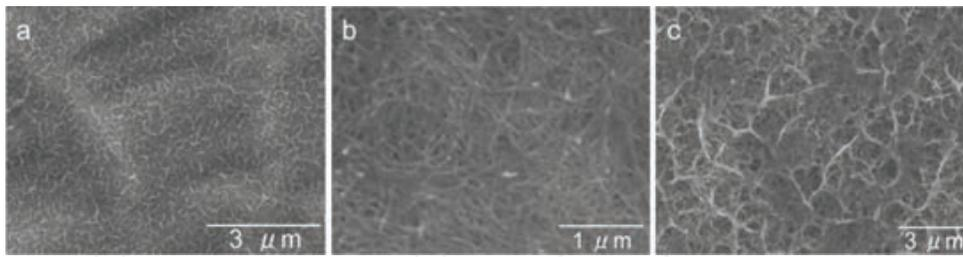
**Figure 9.** SEM images of the sodium titanate nanosheet thin film (a), the sodium titanate nanotube thin film (b) [34], and the sodium titanate thin film with a porous network structure (c) [34] formed on titanium plates.
