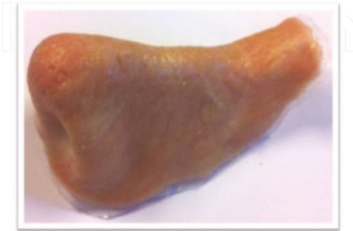
Figure 10. Photograph of a 3D printed nasal prosthesis infiltrated with a compatible medical grade silicone infiltrate (Approx. part Dim: 40 × 24 × 25 mm).
