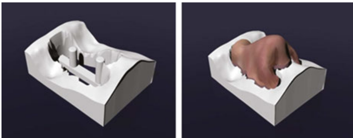
Figure 9. Illustrations demonstrating the design and production of an infiltration bed to support the prosthesis during infiltration with a suitable material (Approx. part Dim: 52 × 36 × 25 mm).
