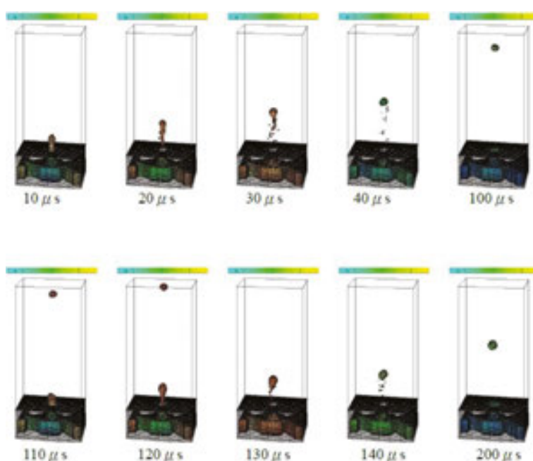
Figure 15. Numerical simulation of DNA in the nozzle diameter 30 \mu\text{m} and 50 \mu\text{m} thickness tapered dual channel injection chamber to 10 kHz operating frequency, three-dimensional side view, in 10, 20, 30, 40, 100, 110, 120, 130, injection of the case 140 and 200 \mu\text{s} .
