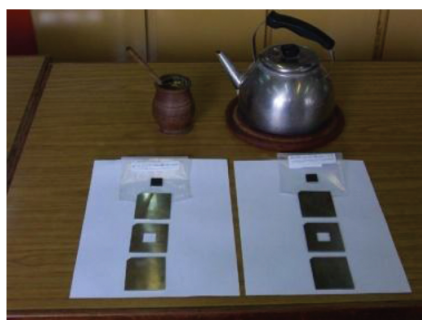
Figure 16. Finished frames, lids and coupons of MZ25 and MZ50 ready to be stacked and welded to conform the two sandwiches.
