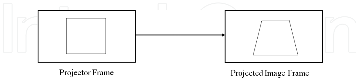
Figure 6. Projected image is distorted when projected onto an oblique surface.
