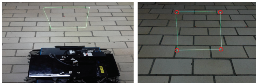
Figure 8. Projection of calibration target and corner extraction.
