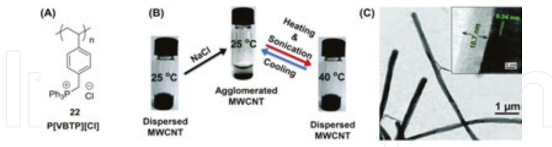
**Figure 17.** (A) Structure of P[VBTP][Cl] **22**. (B) Photographic images showing the dispersion and precipitation of MWNTs in an aqueous solution of **22** in response to addition of NaCl and temperature. (C) TEM image of MWNTs coated with **22**. Adopted from reference [91] with permission.
