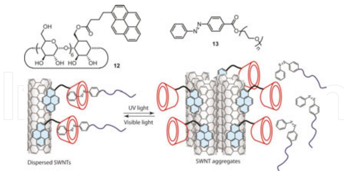
**Figure 9.** Reversible dispersion and release of SWNTs in water using photo-regulated supramolecular guest-host complexation.
