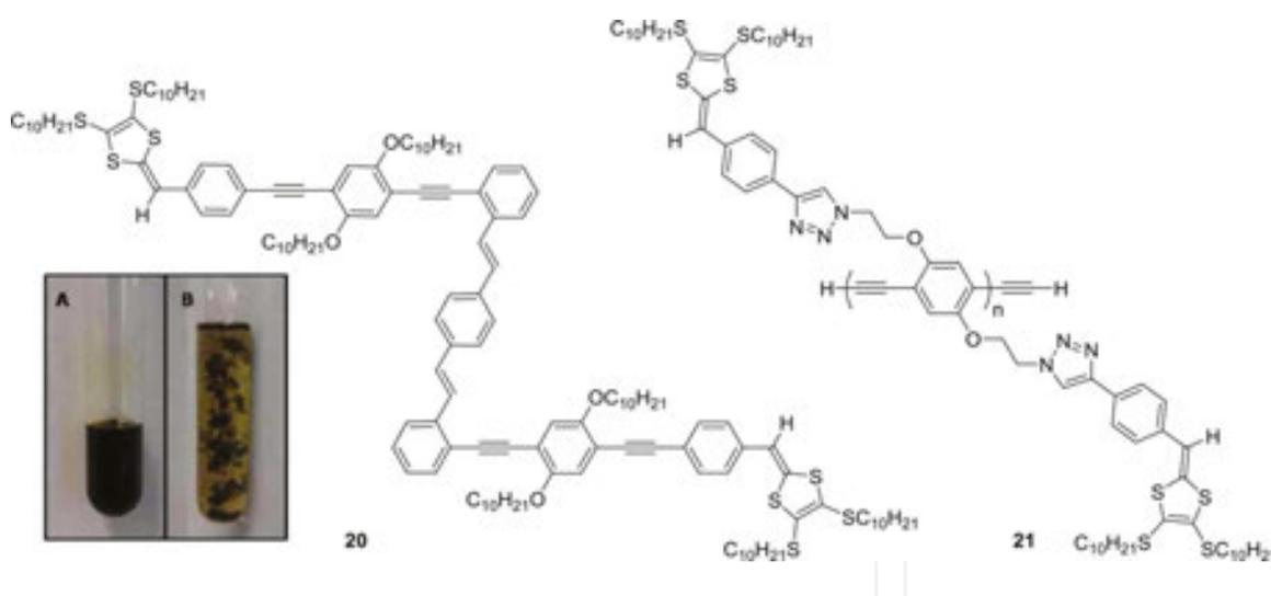
**Figure 14.** Dithiafulvenyl-functionalized conjugated oligomer **20** and polymer **21**. Inset photographic images: (A) SWNTs dispersed in chloroform with **20**, (B) SWNTs released after addition of hexanes.
