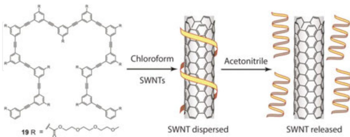
**Figure 13.** Solvent-controlled wrapping and unwrapping of SWNTs with oligo(*m*-phenylene ethynylene) **19**.
