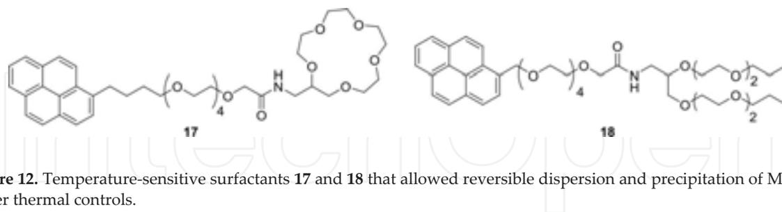
**Figure 12.** Temperature-sensitive surfactants **17** and **18** that allowed reversible dispersion and precipitation of MWNTs under thermal controls.
