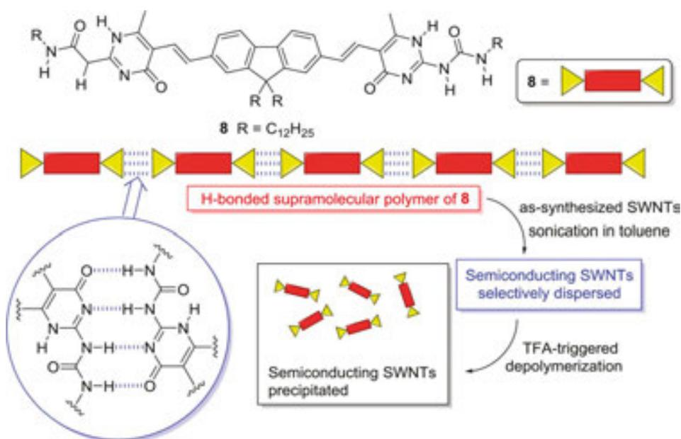
**Figure 6.** Selective dispersion and quantitative release of semiconducting SWNTs using a pH-sensitive H-bonded supramolecular polymer.
