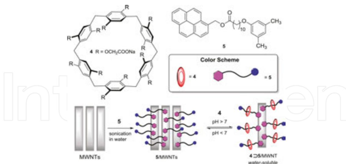
**Figure 4.** Reversible dispersion and release of MWNTs by pH-sensitive guest-host complexation between pillar[6]arene 4 and pyrene derivative 5.
