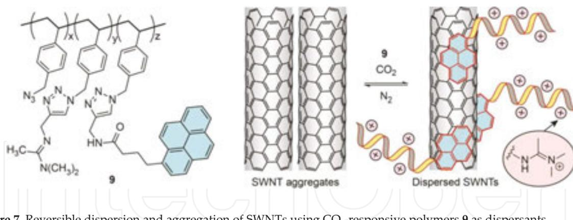
Figure 7. Reversible dispersion and aggregation of SWNTs using  $\text{CO}_2$ -responsive polymers **9** as dispersants.
