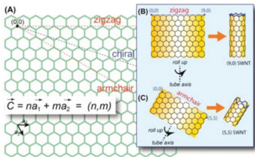
**Figure 1.** (A)–(C) Illustration of the formation of SWNTs with various chiral indices by rolling graphene sheets.
