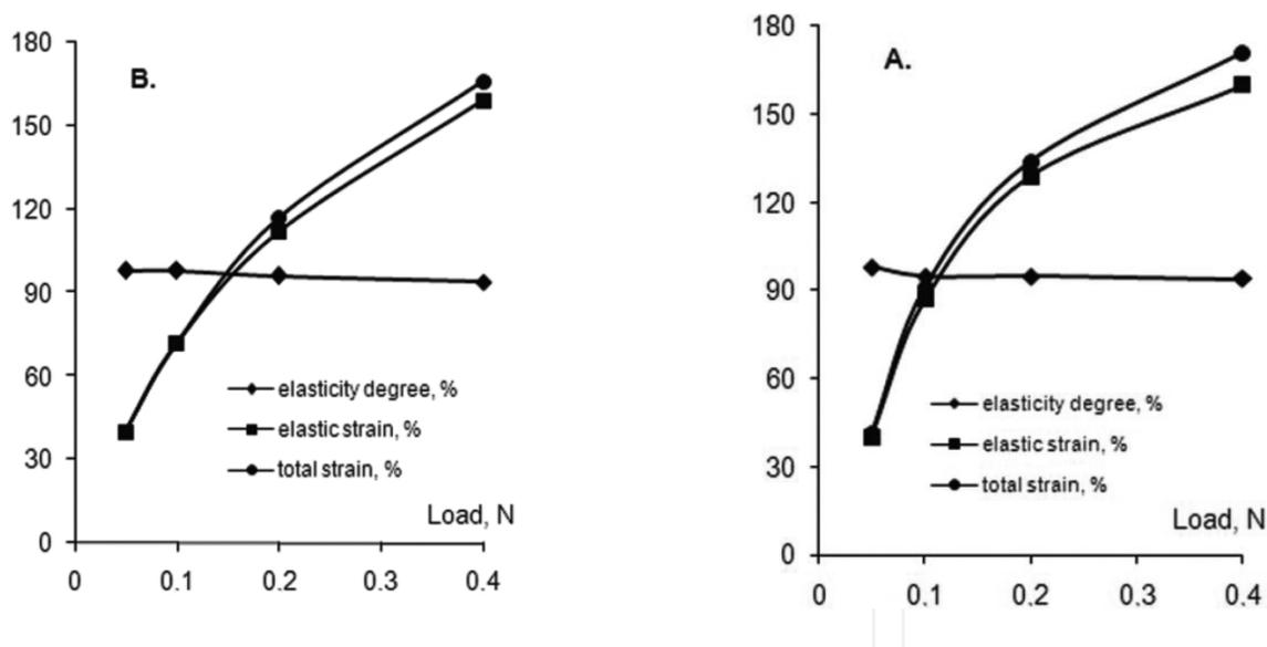
Figure 6. Effect of load on mechanical parameters of Lycra yarn (A) before and (B) after coating with PPy.
