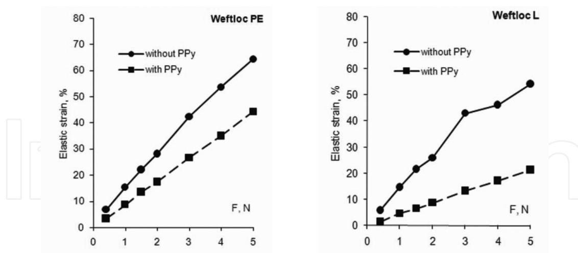
**Figure 8.** Effect of PPy on the elastic strain of Weftloc knitted fabrics in the diagonal direction (loading rate: 200 mm/min).
