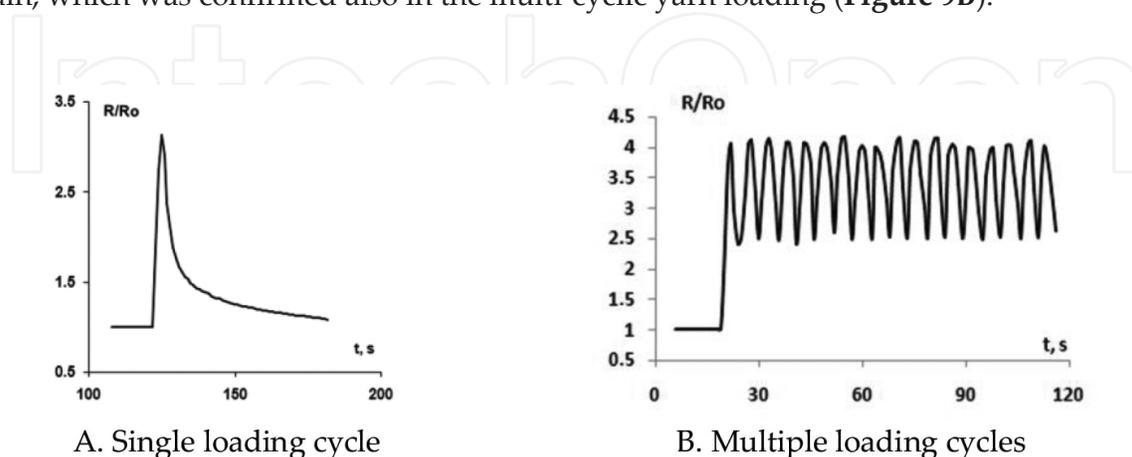
**Figure 9.** Resistance responses of Lycra weft yarn tensioned axially, tensioning rate 50 mm/min, load 8cN. (A) Single loading cycle, (B) multiple loading cycles.
