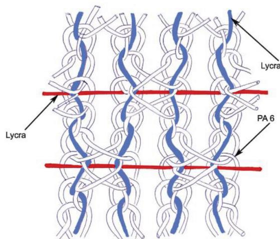
**Figure 1.** Weftloc PE warp knitted fabric.
