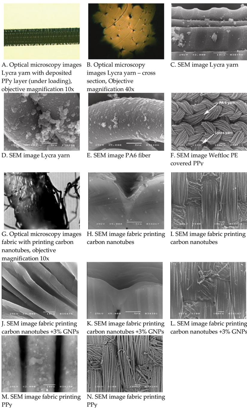
**Figure 4.** SEM and optical microscopy images of: (A–F) PPy coating on Lycra and PA6 yarns and Weftloc PE knitted fabric, (G–I) AquaCyl AQ3001 + cross-linking compound printed on fabric, (J–L) AquaCyl AQ3001 + 3% GNPs + cross-linking compound printed on fabric, (M–N) Polypyrrole + cross-linking compound printed on fabric.
