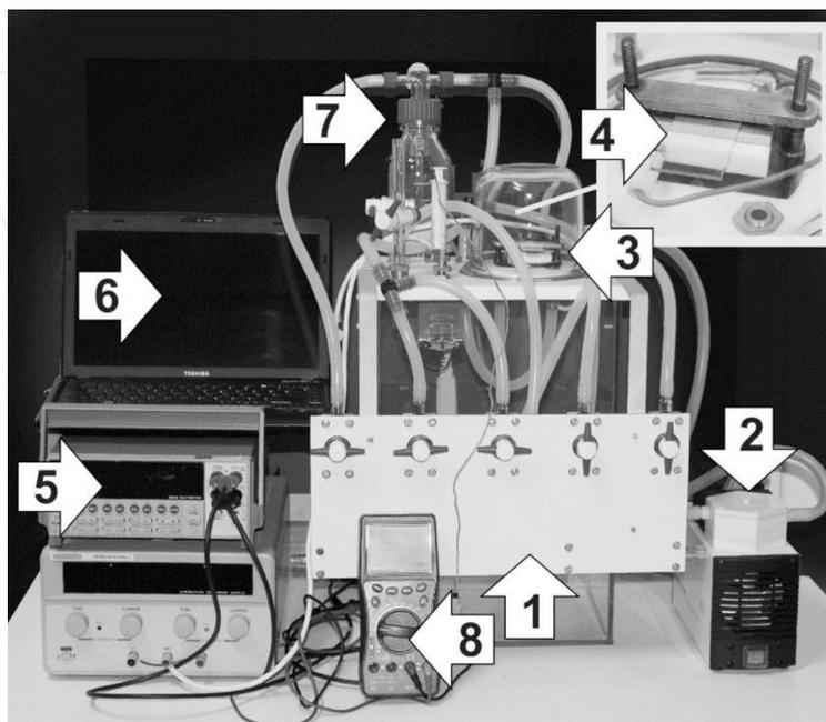
**Figure 3.** Measuring system for investigating the vapor textile sensors: (1) gaseous chamber with the volume of 0.024 m<sup>3</sup>, (2) pump, (3) measurement chamber, (4) measuring electrodes, (5) Keithley multimeter, (6) computer, (7) system ensuring proper humidity of the environment, (8) thermometer [49].
