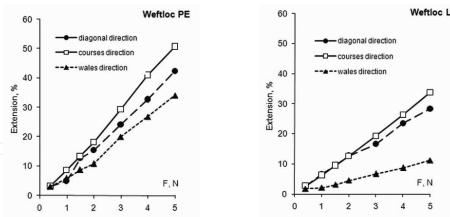
Figure 7. Directional strain of Weftloc fabrics coated with PPy (loading rate: 50 mm/min).
