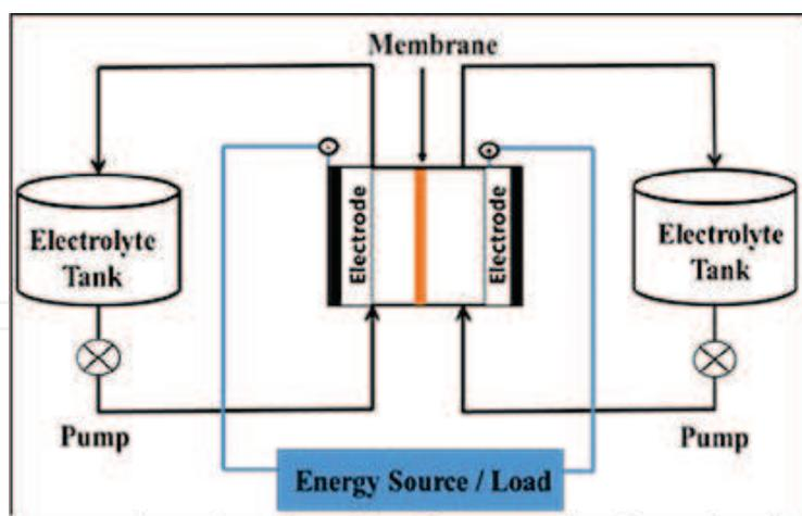
**Figure 7.** Schematic representation of a redox flow battery. The electrolyte is kept in outside tanks and pumped in the two membrane-separated chambers of the active cell.
