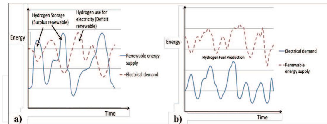
**Figure 5.** Comparison of (a) hydrogen storage for meeting demand when required leaving the system vulnerable to a lack of hydrogen energy available in storage, (b) hydrogen use as a buffer allowing excess hydrogen to be accessed if required.
