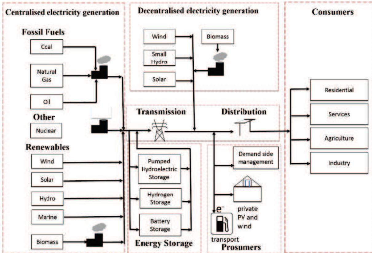
Figure 3. Current energy systems highlighting the dependence on centralised energy generation.
