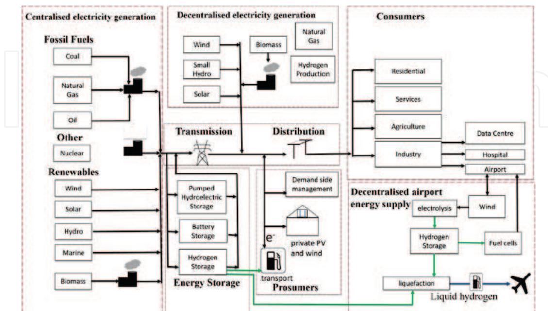
**Figure 8.** Future integrated hydrogen energy systems utilising added value of liquid hydrogen.
