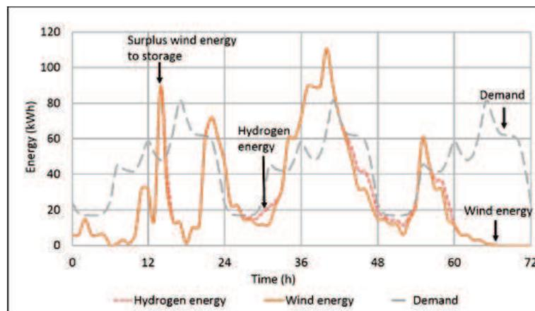
**Figure 6.** Energy versus time diagram for system operation without energy management of hydrogen storage as a buffer. Excess wind energy produces hydrogen for storage; however, not enough hydrogen is available to prevent the requirement of grid energy but reduces curtailment in the system.
