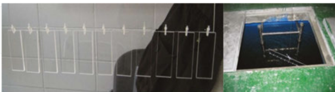
Figure 4. Picture for coupon prepared and set up in the tank.
