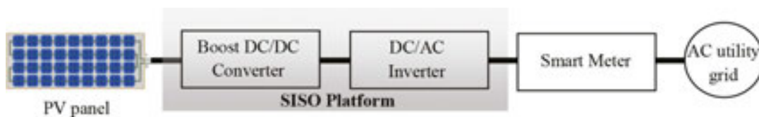
Figure 6. DC source-based SISO platform for grid-tied FIT system.
