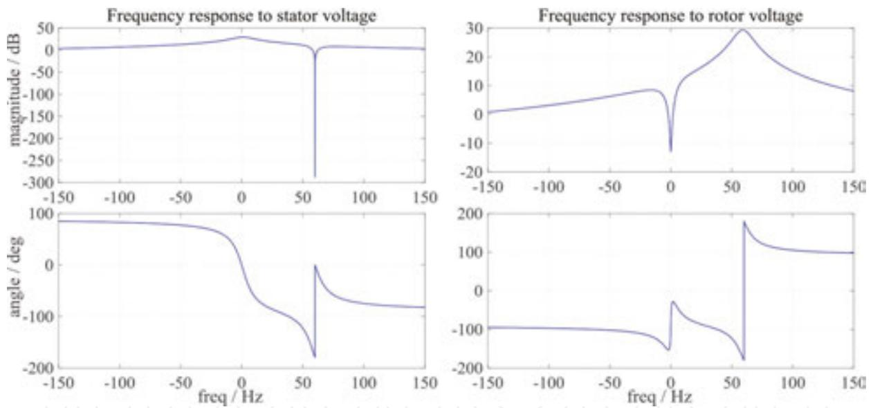
Figure 7. DF IG rotor frequency response.
