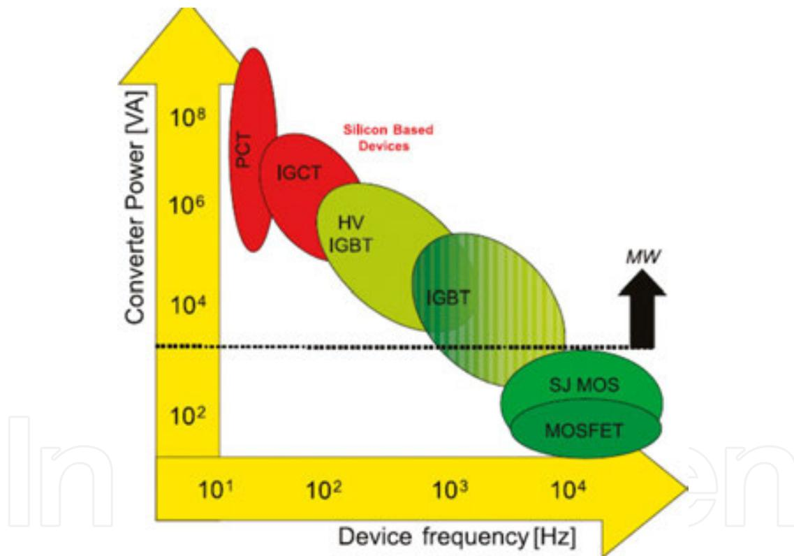
Figure 3. Switching frequency ranges of semiconductor devices [7].
