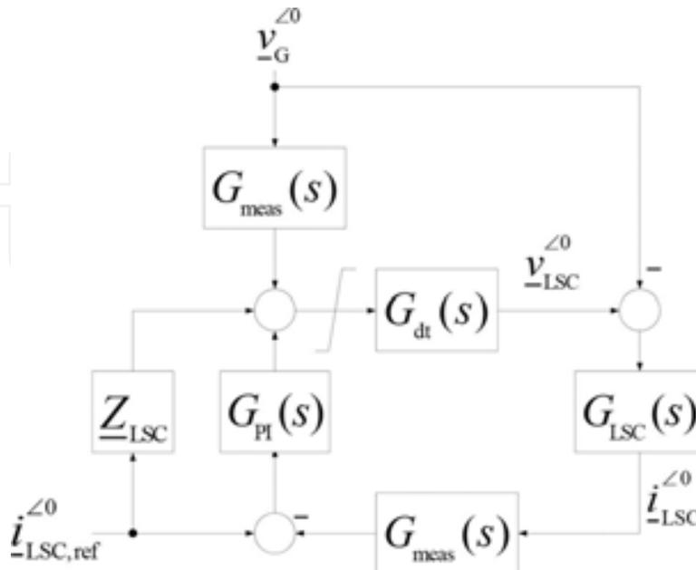
Figure 8. LSC converter inner current control loop.
