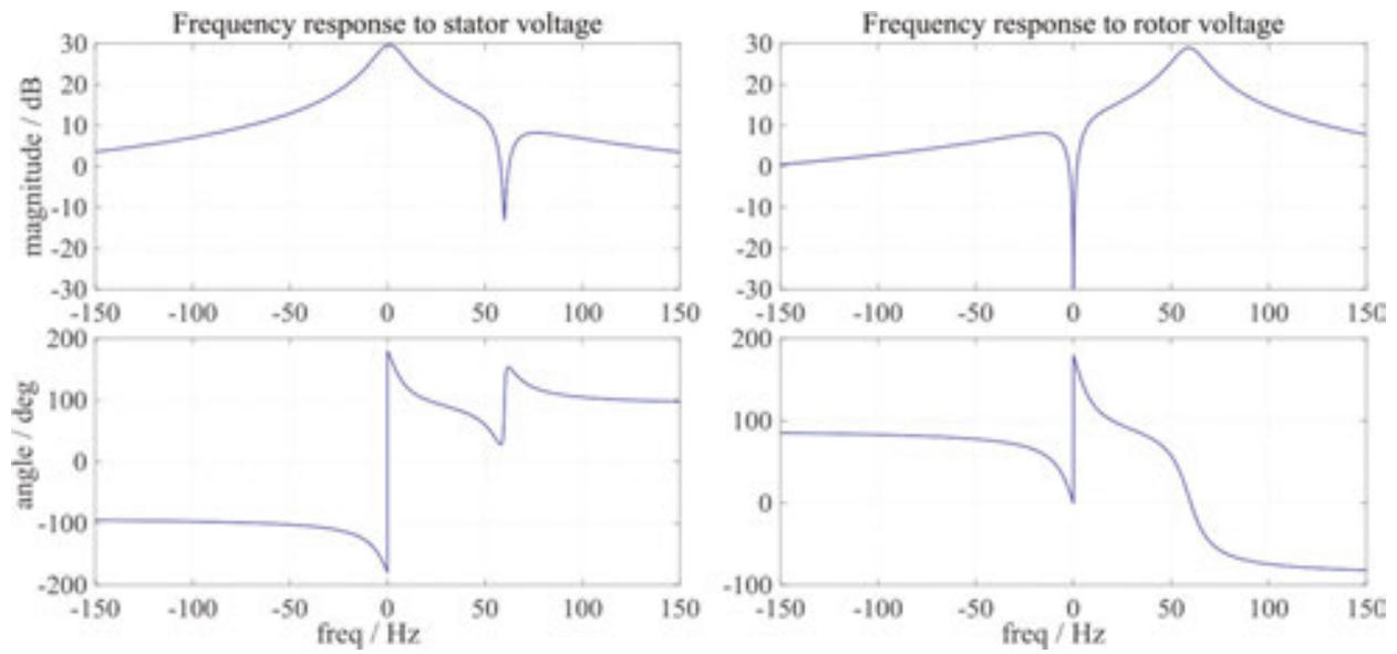
Figure 6. DF IG stator frequency response.
