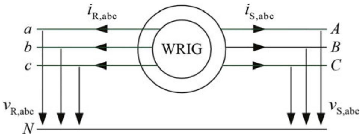
Figure 5. Doubly fed induction generator with measured quantities.
