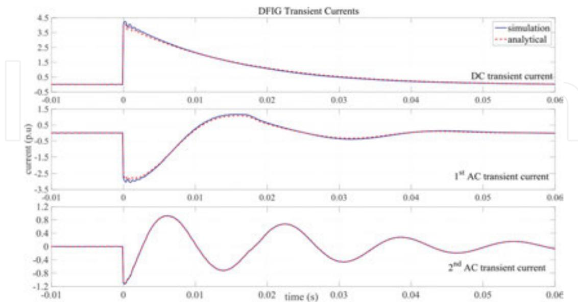
Figure 15. DFIG stator short-circuit current transient components.
