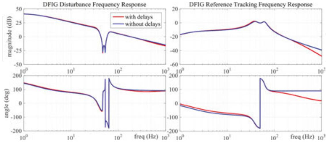
**Figure 13.** Frequency response of DFIG stator current.
