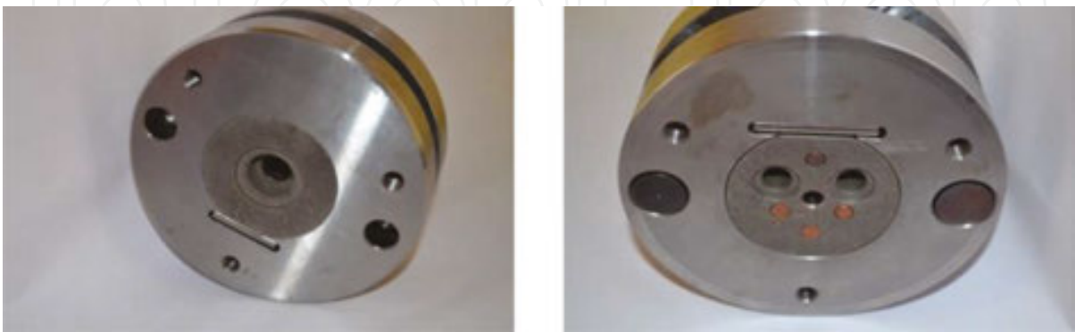
Figure 11. Active elements of moulds made by SLM mounted onto the plates manufactured at Plastor S.A. company from Oradea.
