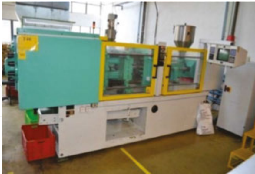
Figure 12. Arburg 370 CMD 800-325 injection moulding equipment (Plastor SA Company Oradea).
