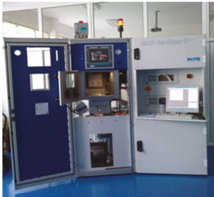
Figure 2. MCP Realizer II SLM 250 system from the Technical University of Cluj-Napoca.
