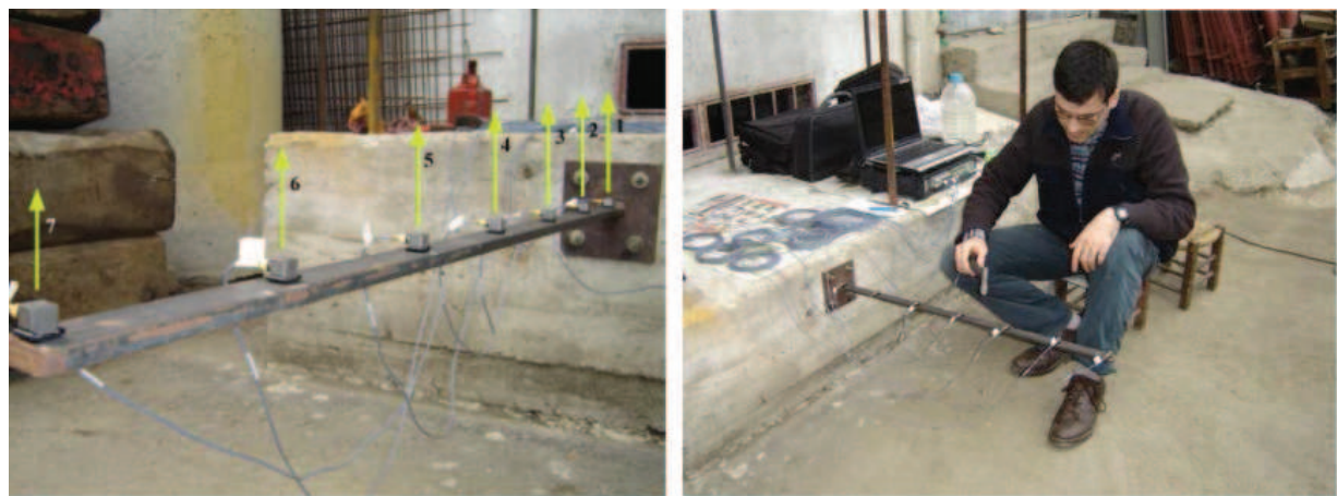
Figure 7. Cantilever beam model, acceleration set-up, and excitation with a hummer.
