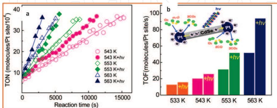
**Figure 11.** (a) Turnover number (TON) for CO oxidation on Pt–CdSe–Pt nanodumbbells with and without light at three different temperatures and (b) TOF for CO oxidation on Pt–CdSe–Pt nanodumbbells with and without light at four different temperatures. During CO oxidation, the TON was measured after a certain amount of time to allow for product molecules to accumulate. Time zero is the point when we started collecting data, not the start of the reaction. Adapted with permission [73].
