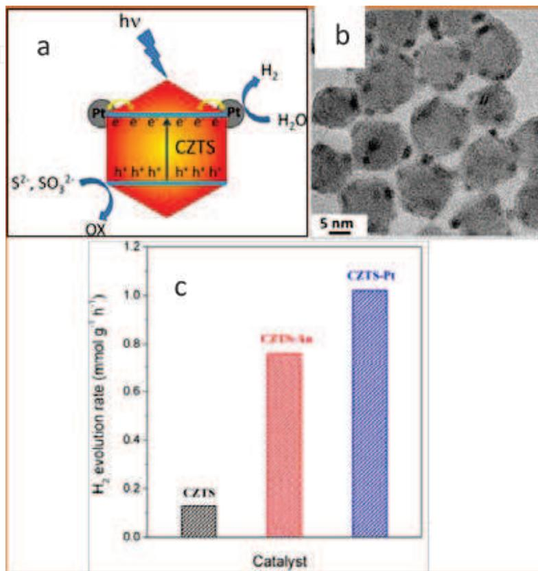
**Figure 15.** (a) Illustration of the possible mechanism of enhancement of the  $\text{H}_2$  evolution rate in CZTS–Pt. (b) HR TEM image of CZTS–Pt heterostructured nanoparticles. (c) Hydrogen evolution rate of CZTS, CZTS–Au, and CZTS–Pt nanomaterials during a 4 h test. Adapted with permission [11].
