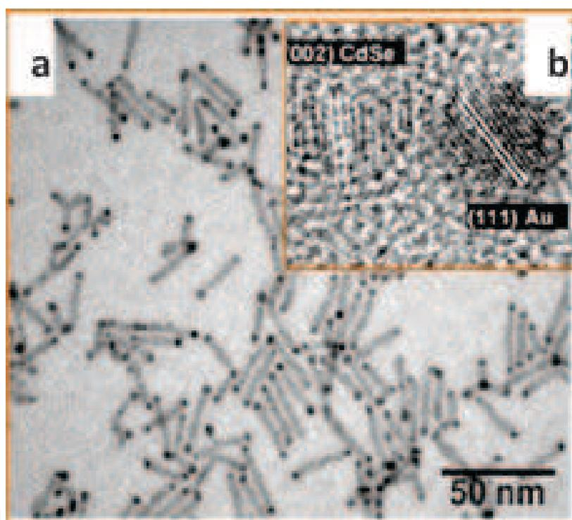
**Figure 1.** (a) CdSe nanorods after Au treatment using AuCl<sub>3</sub>; Au tips are visible. (b) Inset shows HRTEM images of a single Au-tipped CdSe nanorod. The CdSe lattice for the rod in the center and Au tips at the rod edges can be identified, as marked. Adapted with permission [3].
