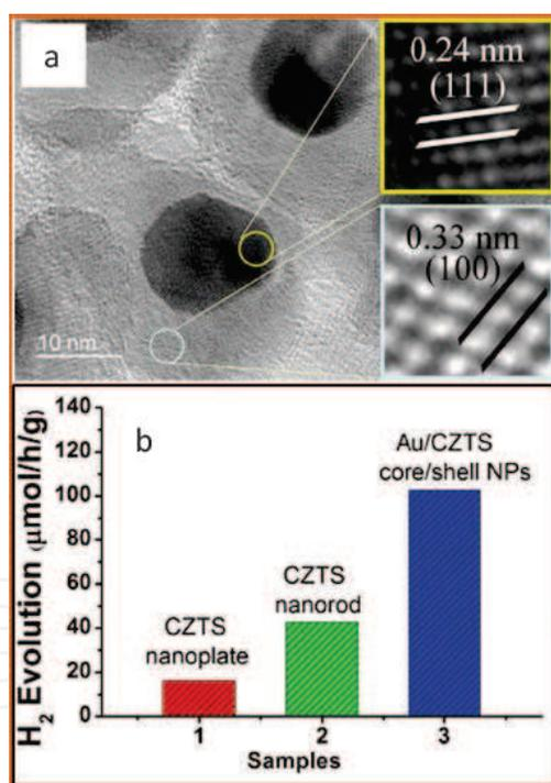
**Figure 14.** (a) Typical TEM and high-resolution TEM image of as-prepared Au/CZTS core/shell NPs. (b) A Plot comparing the photocatalytic H<sub>2</sub> evolution among CZTS nanoplates (red), CZTS nanorods (green), and Au/CZTS core/shell NPs (blue). Adapted with permission [31].
