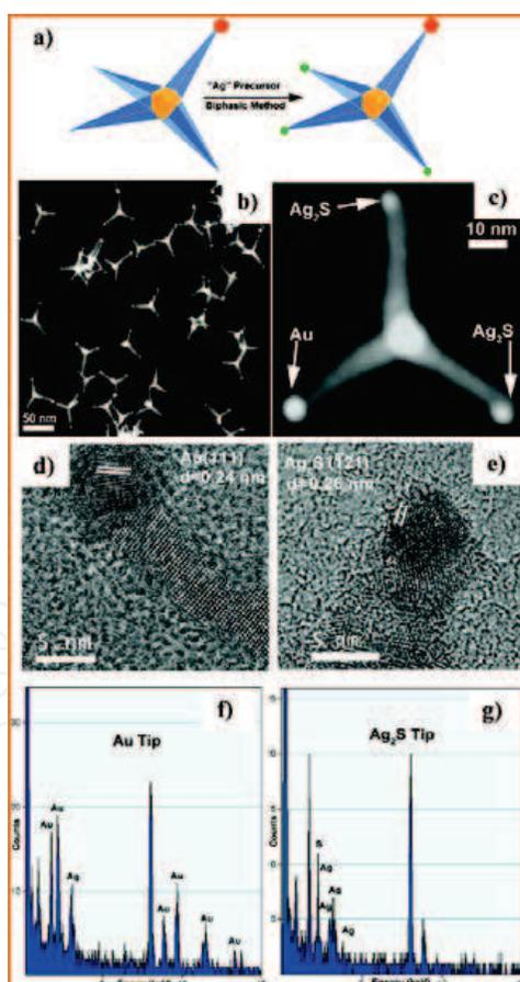
**Figure 6.** (a) Reaction schematic to obtain hierarchically complex CdSe-seeded CdS tetrapods with Au at precisely one tip and Ag<sub>2</sub>S at the other three. (b) Representative HAADF-STEM image of tetrapods with cone-like arms fabricated according to the strategy shown in a. (c) Magnified view of one of the tetrapods in b, with the different tips labeled. (d, e) HRTEM images of the different tetrapod arm tips showing the visible lattice fringes of the Ag<sub>2</sub>S (1021) and Au (111)
