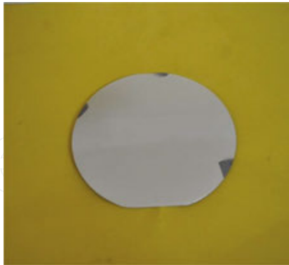
Figure 14. Photograph of platinum thin film deposited on oxidized three-inch-silicon wafer by RF sputtering technique.
