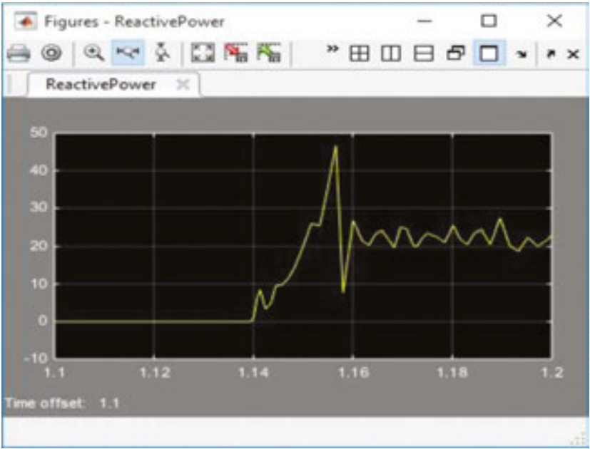
Figure 10. Reactive power variation on coil at connecting.
