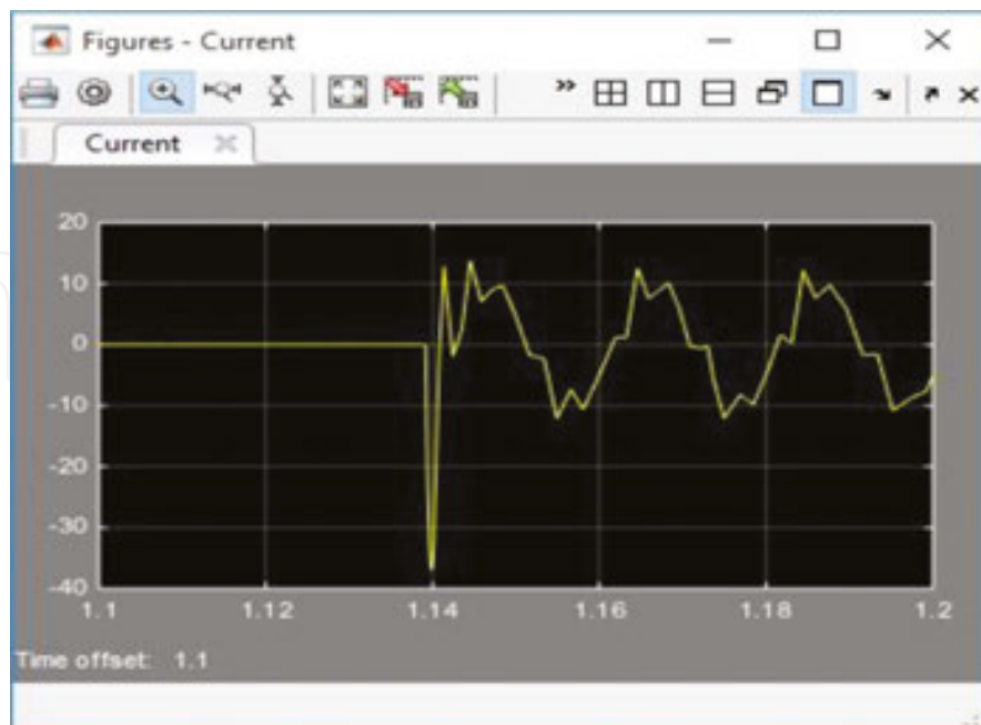
Figure 8. Current variation on coil at connecting.
