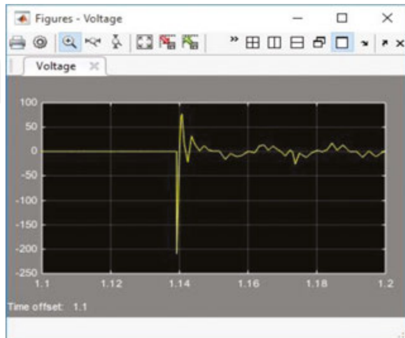
Figure 7. Voltage variation on coil when connection is initiated.
