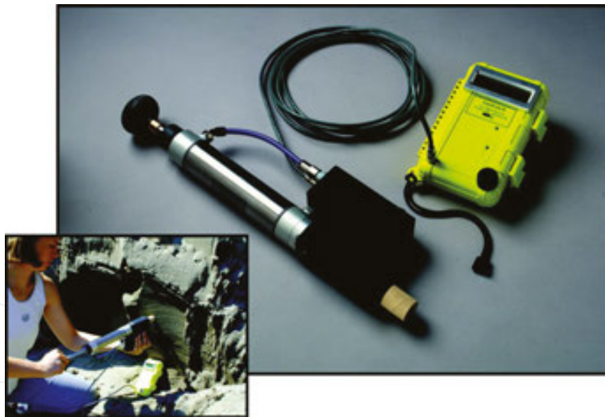
Figure 5. Tiny Perm (New England Research Inc.) taken with the permission from Brown and Smith [40].
