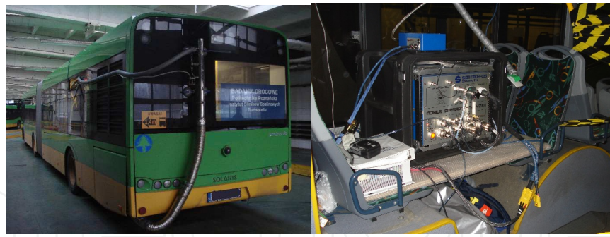
Figure 1. City bus with the measurement equipment fitted during the road tests
