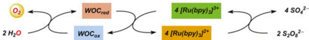
Figure 5. Three-component system for light-driven water oxidation consisting of a water oxidation catalyst, a [\text{Ru}(\text{bpy})_3]^{2+} -type photosensitizer and persulfate as the sacrificial electron acceptor.
