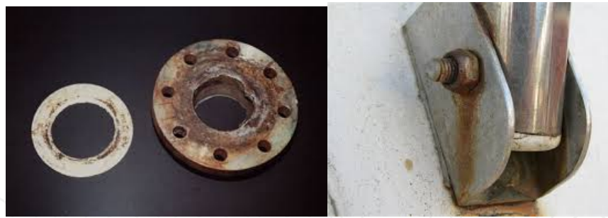
Figure 4. (a) Crevice Corrosion on a Steel Flange [17] and (b) Typical View of Crevice Corrosion.
