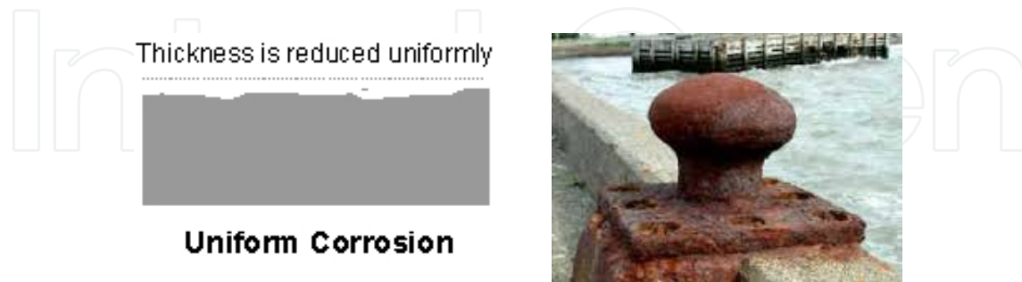
Figure 3. (a) Schematic Representation of Uniform Corrosion and (b) a Weathering Steel [16].
