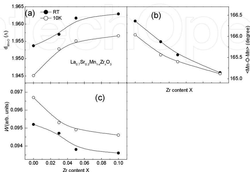
**Figure 6.** Average Mn-O bond lengths (a), Mn-O-Mn bond angles (b), and electronic bandwidth parameter  $W$ , of  $\text{La}_{0.7}\text{Sr}_{0.3}\text{Mn}_{1-x}\text{Zr}_x\text{O}_3$  ( $x = 0.0, 0.03, 0.05, 0.10$ ) at room temperature and at 10K.
