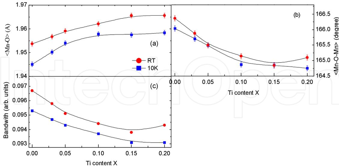
**Figure 3.** Average Mn-O bond lengths (a), Mn-O-Mn bond angles (b), and electronic bandwidth parameter  $W$  (c), of  $\text{La}_{0.7}\text{Sr}_{0.3}\text{Mn}_{1-x}\text{Ti}_x\text{O}_3$  at room temperature and at 10K.
