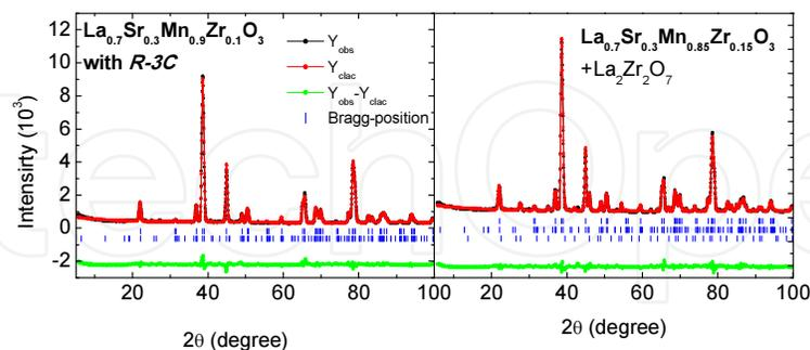
**Figure 5.** Neutron diffraction patterns of  $\text{La}_{0.7}\text{Sr}_{0.3}\text{Mn}_{0.9}\text{Zr}_{0.1}\text{O}_3$  and  $\text{La}_{0.7}\text{Sr}_{0.3}\text{Mn}_{0.85}\text{Zr}_{0.15}\text{O}_3$  at room temperature.
