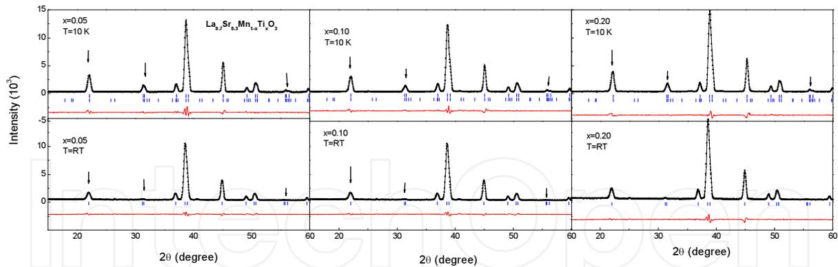
**Figure 1.** ND patterns of  $\text{La}_{0.7}\text{Sr}_{0.3}\text{Mn}_{1-x}\text{Ti}_x\text{O}_3$  ( $x = 0.05, 0.10, 0.20$ ) at RT and 10 K. (The bottom curves (red line) are the difference between experimental data and the refinement data. The vertical bars (blue line) represent the magnetic (bottom) and Bragg (top) peak positions). Arrows shows some of the major magnetic diffraction peaks.
