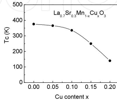
**Figure 9.** The Curie temperature of  $\text{La}_{0.7}\text{Sr}_{0.3}\text{Mn}_{1-x}\text{Cu}_x\text{O}_3$ .
