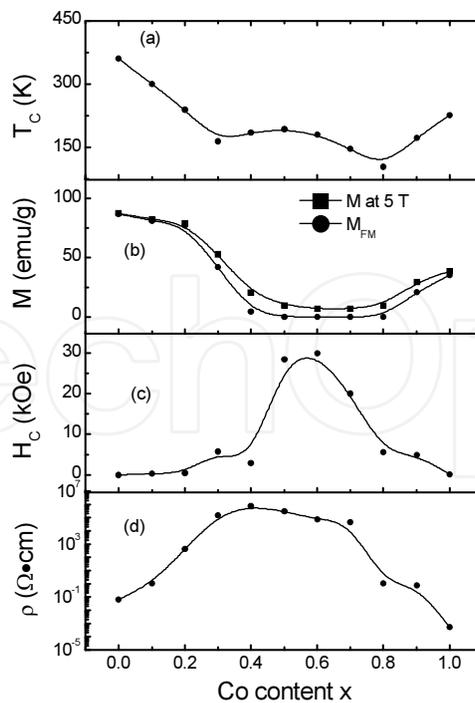
**Figure 14.** (a) Curie temperature ( $T_C$ ), (b) the magnetization at the field of 5 T and the ferromagnetic component extracted from the M-H curve, (c) the coercivity at 5 K, (d) the resistivity at 70 K of  $\text{La}_{0.7}\text{Sr}_{0.3}\text{Mn}_{1-x}\text{Co}_x\text{O}_3$ .
