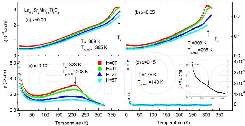
**Figure 4.** The temperature dependent resistivity for  $\text{La}_{0.7}\text{Sr}_{0.3}\text{Mn}_{1-x}\text{Ti}_x\text{O}_3$  compounds ( $x = 0.0$ (a),  $0.05$ (b),  $0.10$ (c), and  $0.15$ (d)) under magnetic field  $H = 0, 1, 3,$  and  $5\text{ T}$ . Arrows indicate the resistivity maximum temperature  $T_{\rho,\text{max}}$ . The inset in (d) is the plot of resistivity of  $x = 0.15$  compound (with log scale) in  $H = 0\text{ T}$ .
