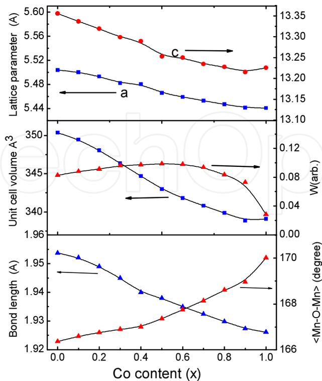
**Figure 12.** The lattice parameters  $a$ ,  $c$ , unit cell volume, bandwidth  $W$ , bond length  $d_{\text{Mn-O}}$  and bond angle  $\langle \text{Mn-O-Mn} \rangle$  for  $\text{La}_{0.7}\text{Sr}_{0.3}\text{Mn}_{1-x}\text{Co}_x\text{O}_3$  at RT.
