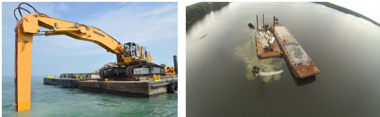
Figure 1. Mechanical dredges (U.S. Army Corps of Engineers – Downloaded from www.flickr.com )
