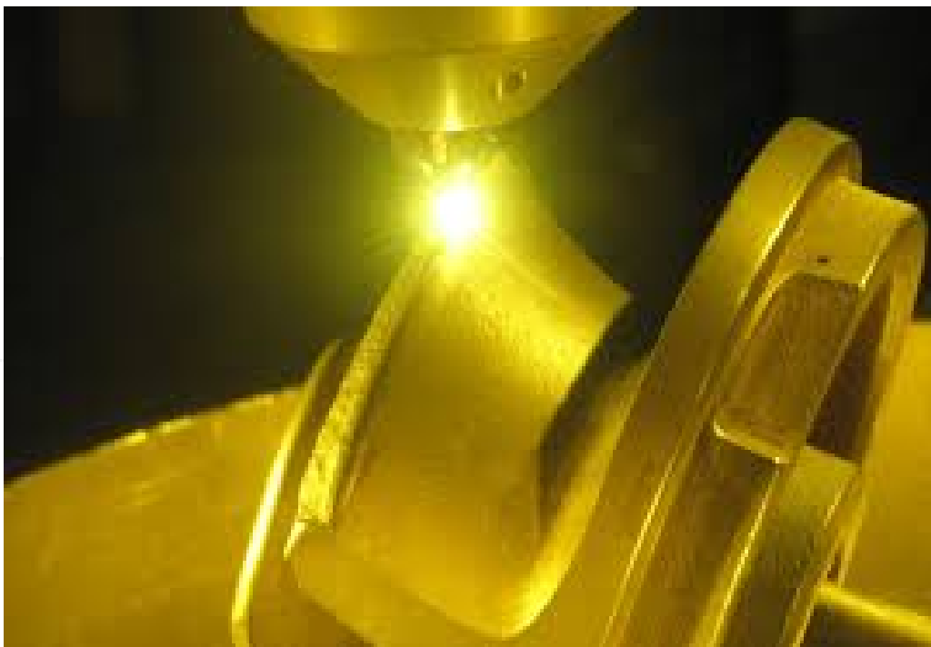
Figure 8. Fabrication of impeller pump using LENS™ [40].
