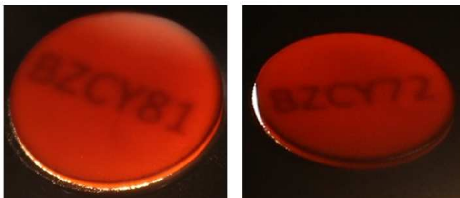
Figure 10. BZCY81 and BZCY72 specimens after NiO extraction at 1600 °C, followed by annealing in H 2 . At 800 °C for 24 hrs.
