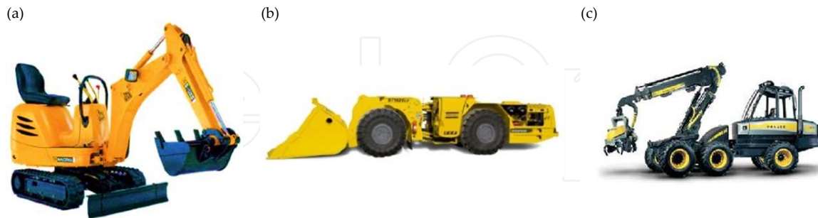
Figure 1. Examples of non-road mobile machinery: (a) excavator; (b) mine loader and (c) forest harvester.
