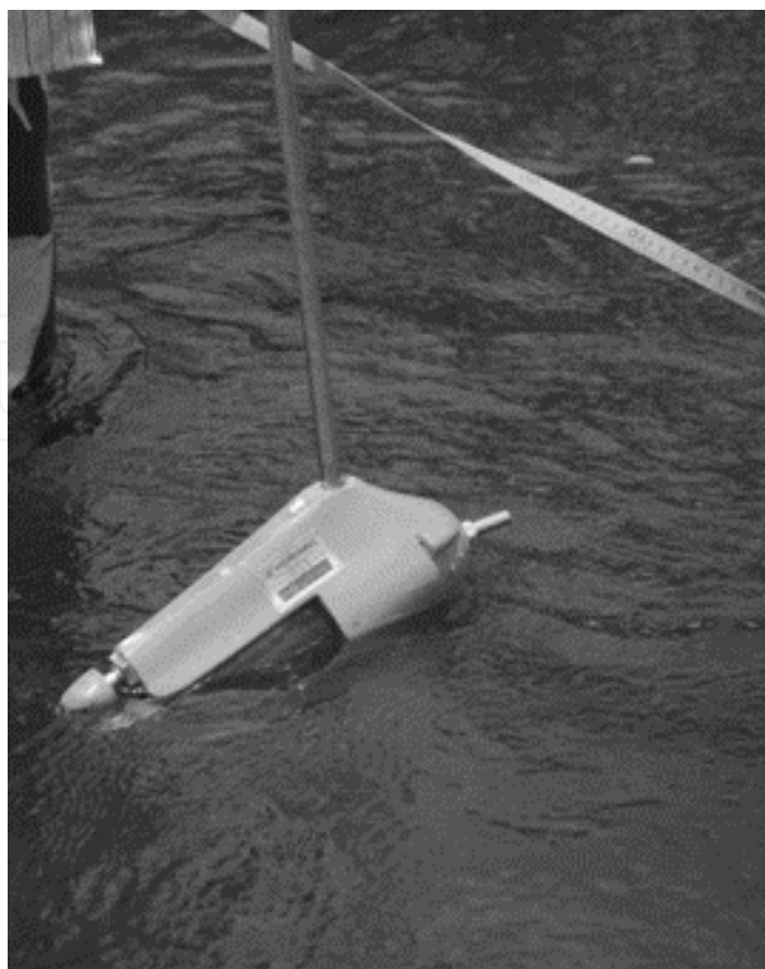
Figure 3. Suspended sediment sampling (sampler - US DH-48) in the Capibaribe River.
