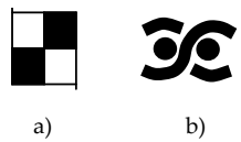
Figure 10. The first effect or ground fabric is created by the warp (black) and weft (black) in plain weave; a) weave unit; b) cross section in the weft direction
