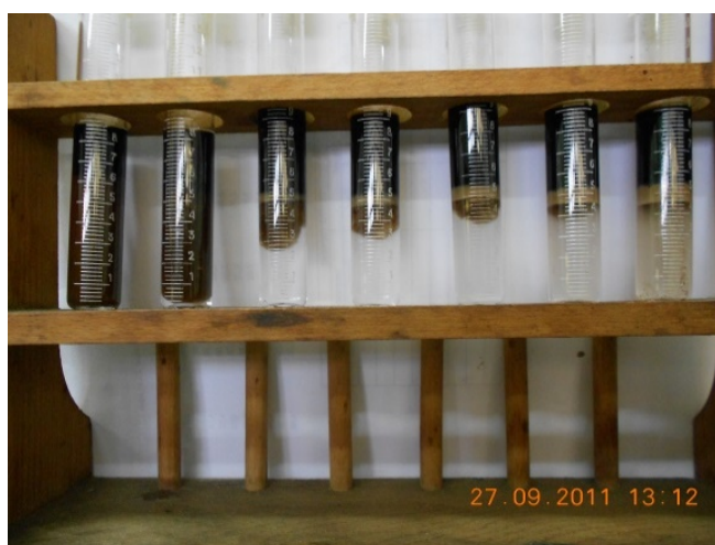
Figure 3. Stability bottle test of water-in-crude-oil emulsion (Silva, 2012).
