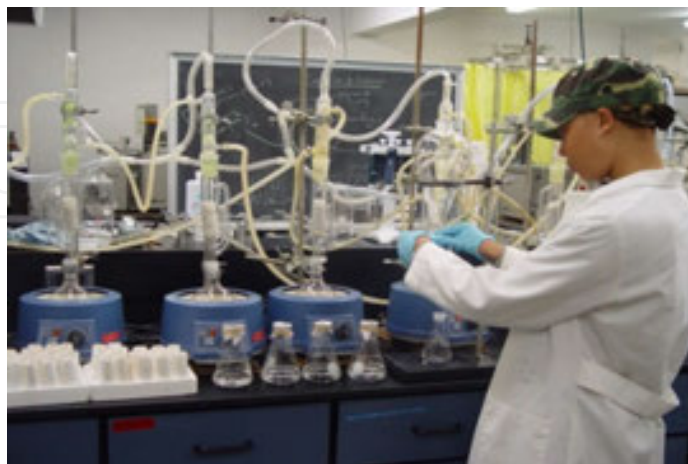
Figure 13. Use of soxhlet extraction units and liquid-liquid partition for extraction of dimethazone and trifluralin herbicides from soil.
