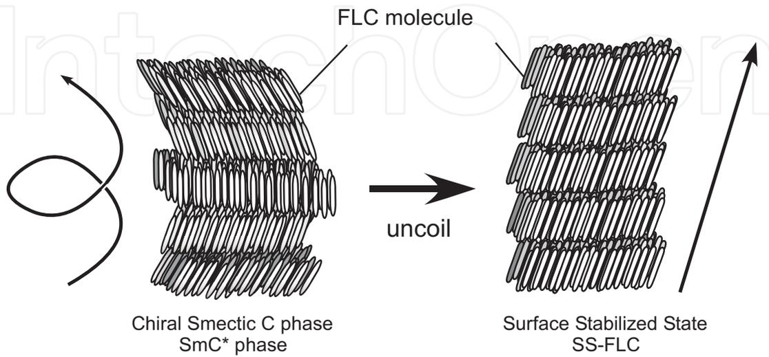
Figure 5. Structures of the SmC phase and the SS-state of the SmC phase (SS-FLC).
