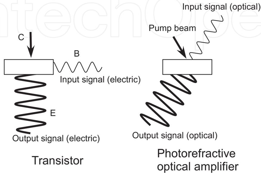
Figure 1. Transistor in electric circuit and photorefractive amplifier.
