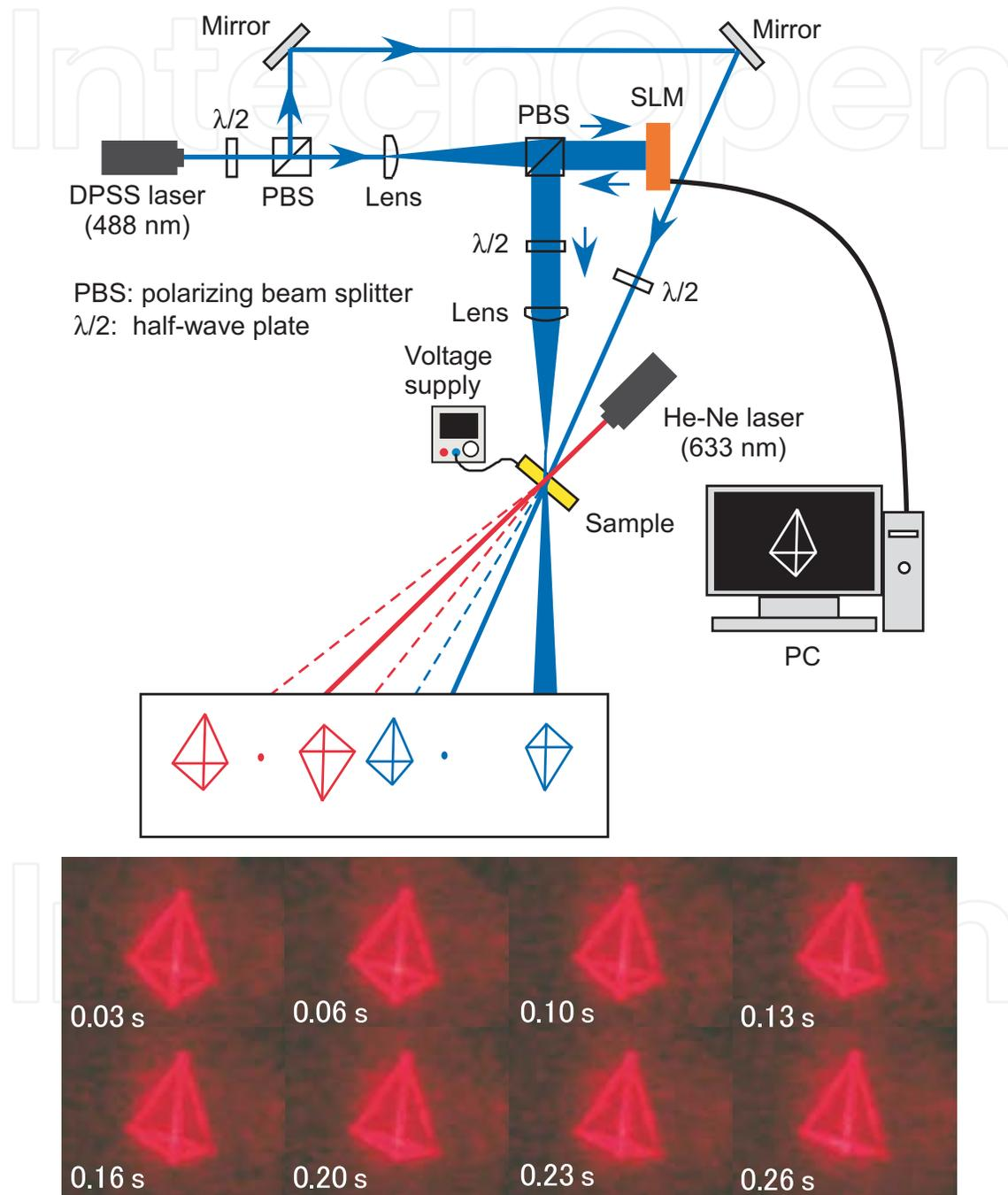
**Figure 29.** Dynamic hologram formation experiment on an FLC sample. A computer-generated animation was displayed on the SLM. The SLM modulated the object beam (488 nm), which was irradiated on the FLC sample and allowed to interfere with the reference beam. The readout beam (633 nm) was irradiated on the FLC and diffraction was observed.
