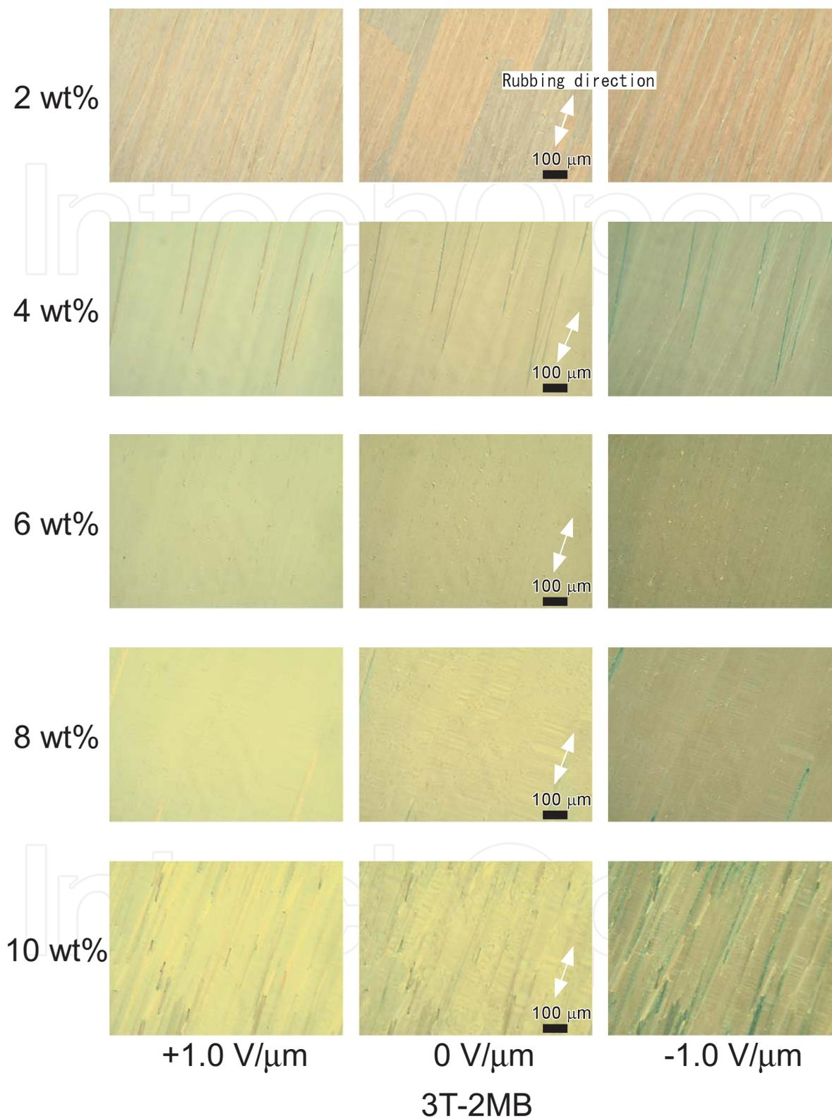
**Figure 18.** Textures of FLC mixtures containing 3T-2MB in a 10  $\mu\text{m}$  gap LC cell observed under a polarizing microscope. The strengths of the external electric field were +1.0, 0, and 1.0 V/ $\mu\text{m}$ . The direction of the applied electric field is shown in Fig. 5. The 3T-2MB concentrations were in the range of 2 wt.% to 10 wt.% with the addition of 0.1 wt.% TNF.
