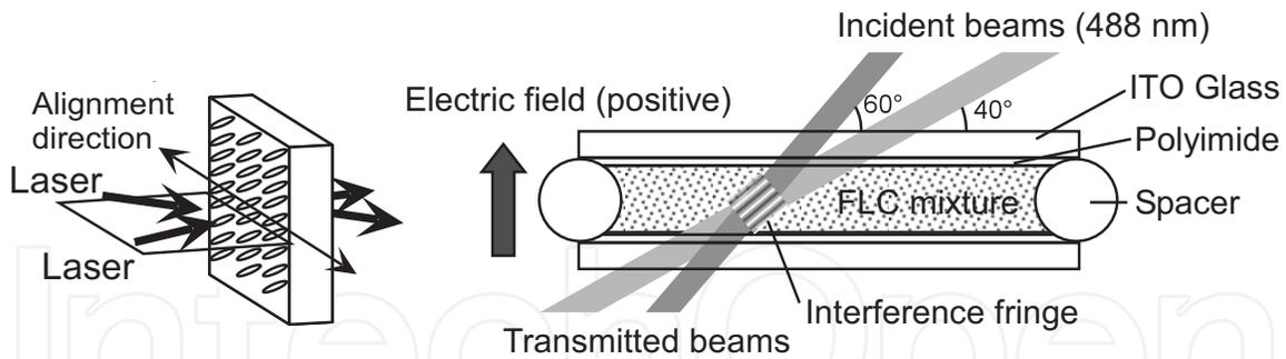
Figure 11. Laser beam incidence condition and the structure of the LC cell.
