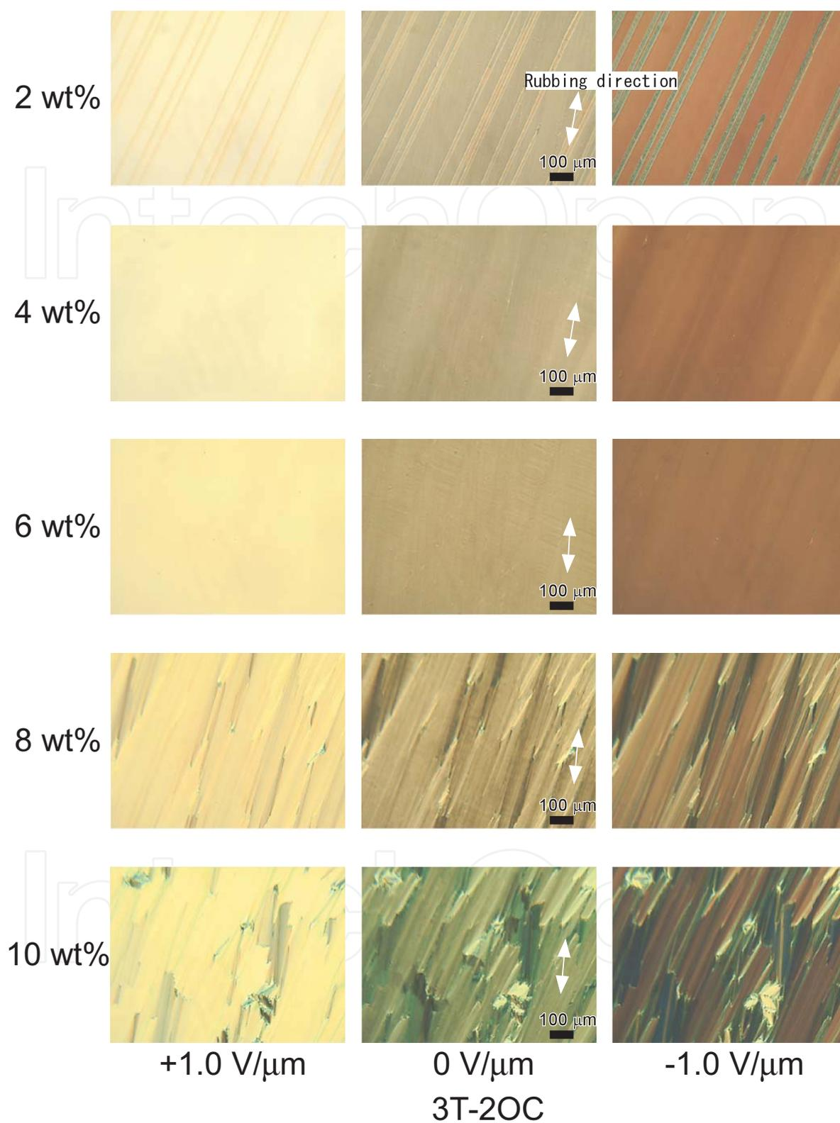
**Figure 19.** Textures of FLC mixtures containing 3T-2OC in a 10  $\mu\text{m}$  gap LC cell observed under a polarizing microscope. The strengths of the external electric field were +1.0, 0, and 1.0 V/ $\mu\text{m}$ . The direction of the applied electric field is shown in Fig. 5. The 3T-2OC concentrations were in the range of 2 wt.% to 10 wt.% with the addition of 0.1 wt.% TNF.
