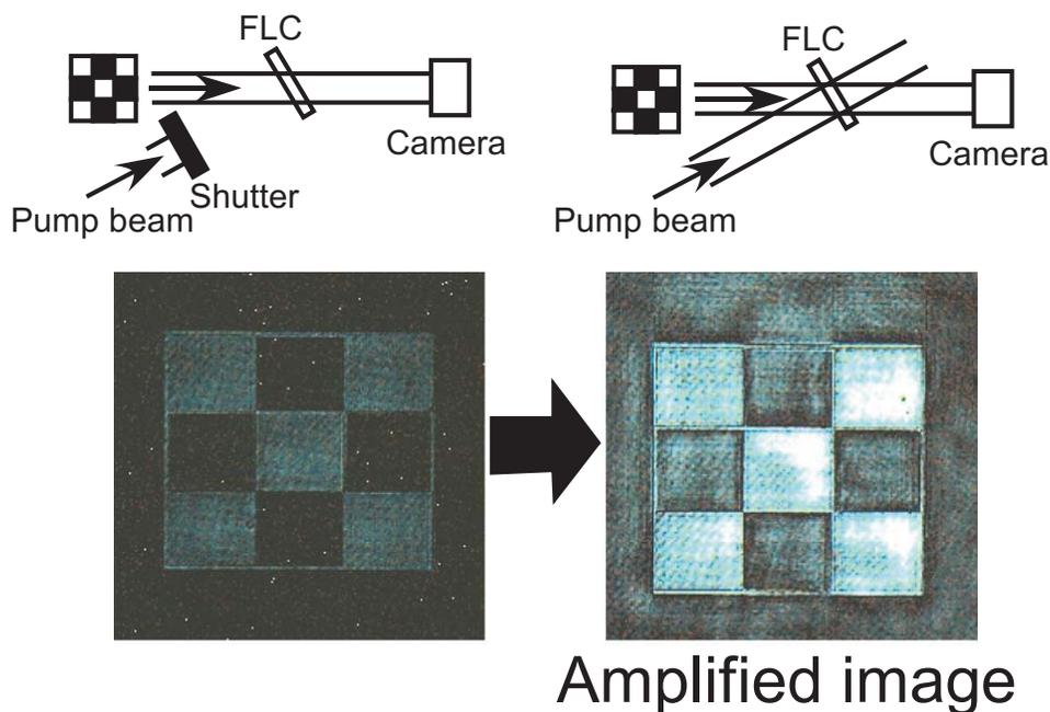
**Figure 26.** Optical image amplification experiment. A computer-generated image was displayed on the SLM. The SLM modulated the object beam (473 nm), which was irradiated on the FLC sample and interfered with the pump beam. The image transmitted through the FLC sample (10 wt.% 3T-2MB) was monitored with a CCD camera.
