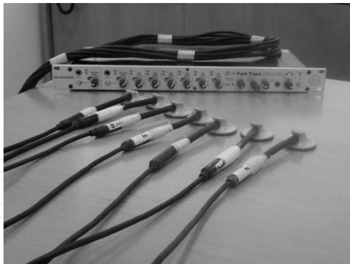
Figure 2. Multi-channel equipment for computerised respiratory sound analysis.
