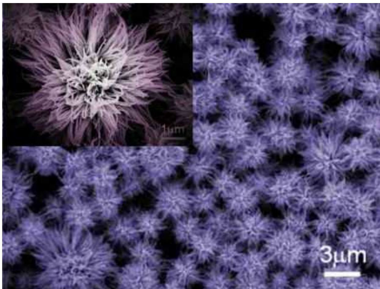
Figure 7. SEM images of Bi_2S_3 nanoflowers synthesized using BiCl_3 and CH_3CSNH_2 as the precursors and [BMIM][BF_4] as the solvent and template [69].
