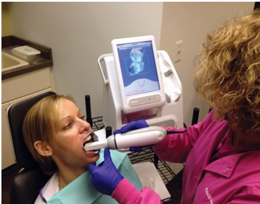
Figure 5. The Lythos™ Digital Impression System [36]
