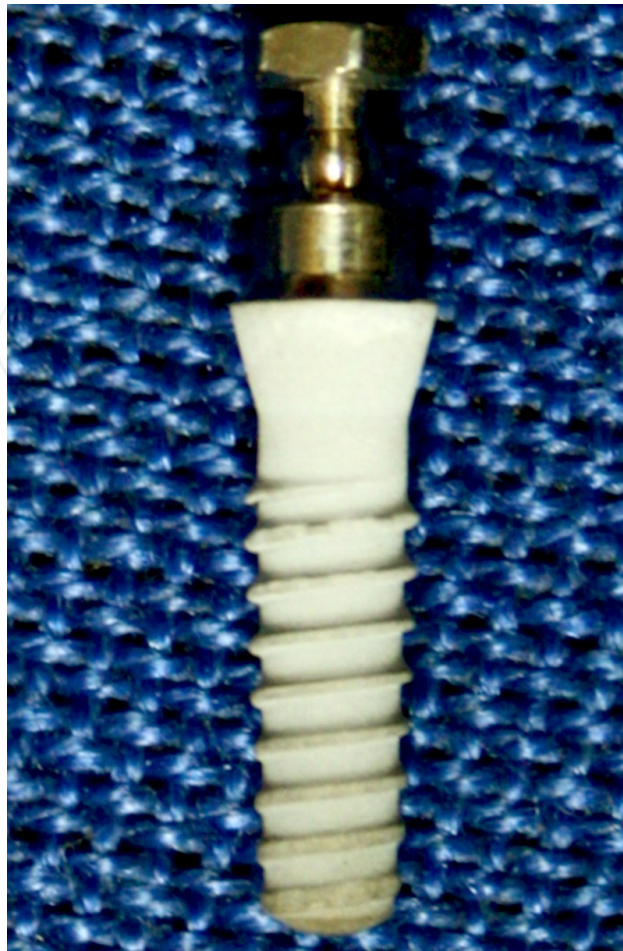
Figure 7. Hydroxyapatite-coated titanium implant.
