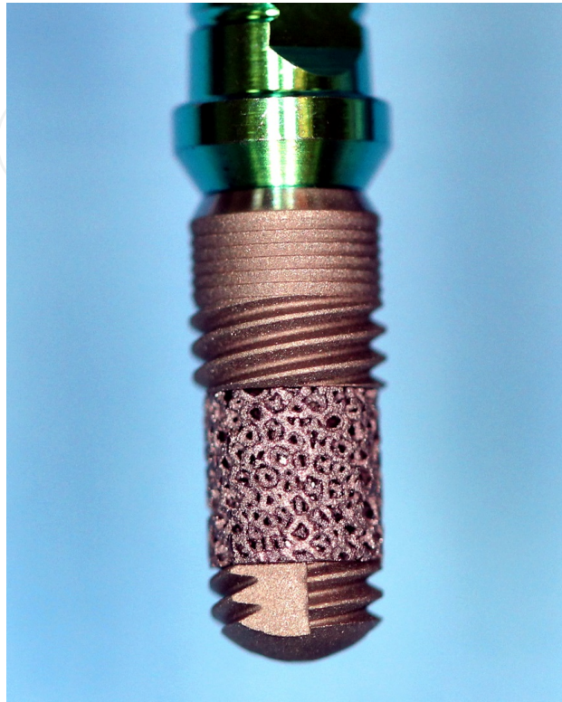
Figure 8. A trabecular implant that could be used to load drugs.
