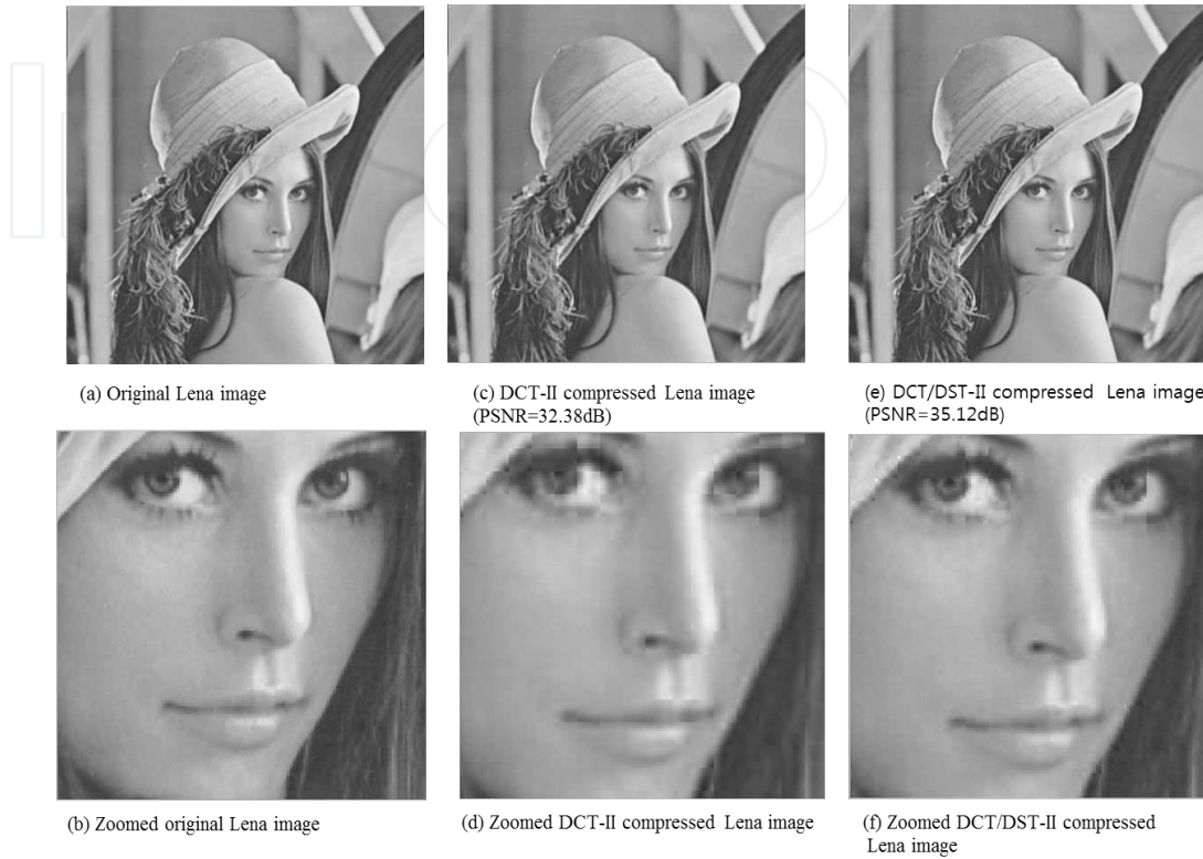
Figure 5. Image Coding Results showing DCT-II only and jointly optimized DCT/DST-II compression (a) Original Lena image (b) zoomed original Lena image (c) DCT-II compressed Lena image(PSNR=32.38 dB) (d) Zoomed DCT-II compressed Lena image (e) DCT/DST-II compressed Lena image (PSNR=35.12 dB) (f) Zoomed DCT/DST-II compressed Lena image.
