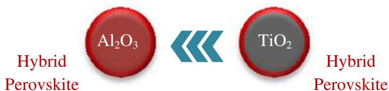
Figure 17. Switching \text{TiO}_2 to an \text{Al}_2\text{O}_3 in Gratzel perovskites solar cell
