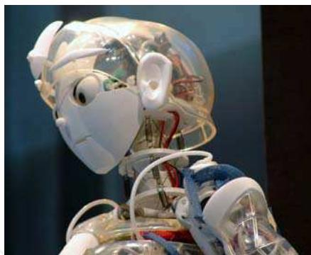
Fig. 10. Muscle-driven head for multi-modal communication.
