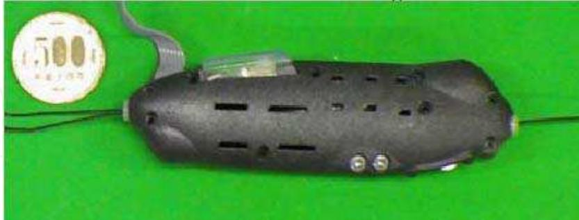
Fig. 2. A newly-developed, sensors-integrated muscle unit.
