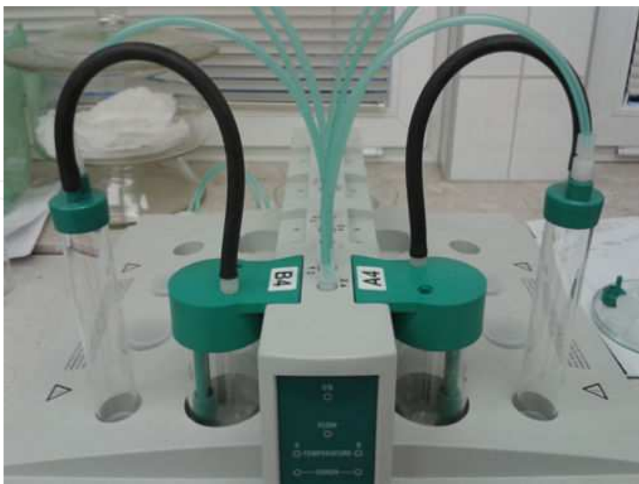
Figure 31. A test assembly for oxidation stability tests according to EN 15751 (Rancimat method).
