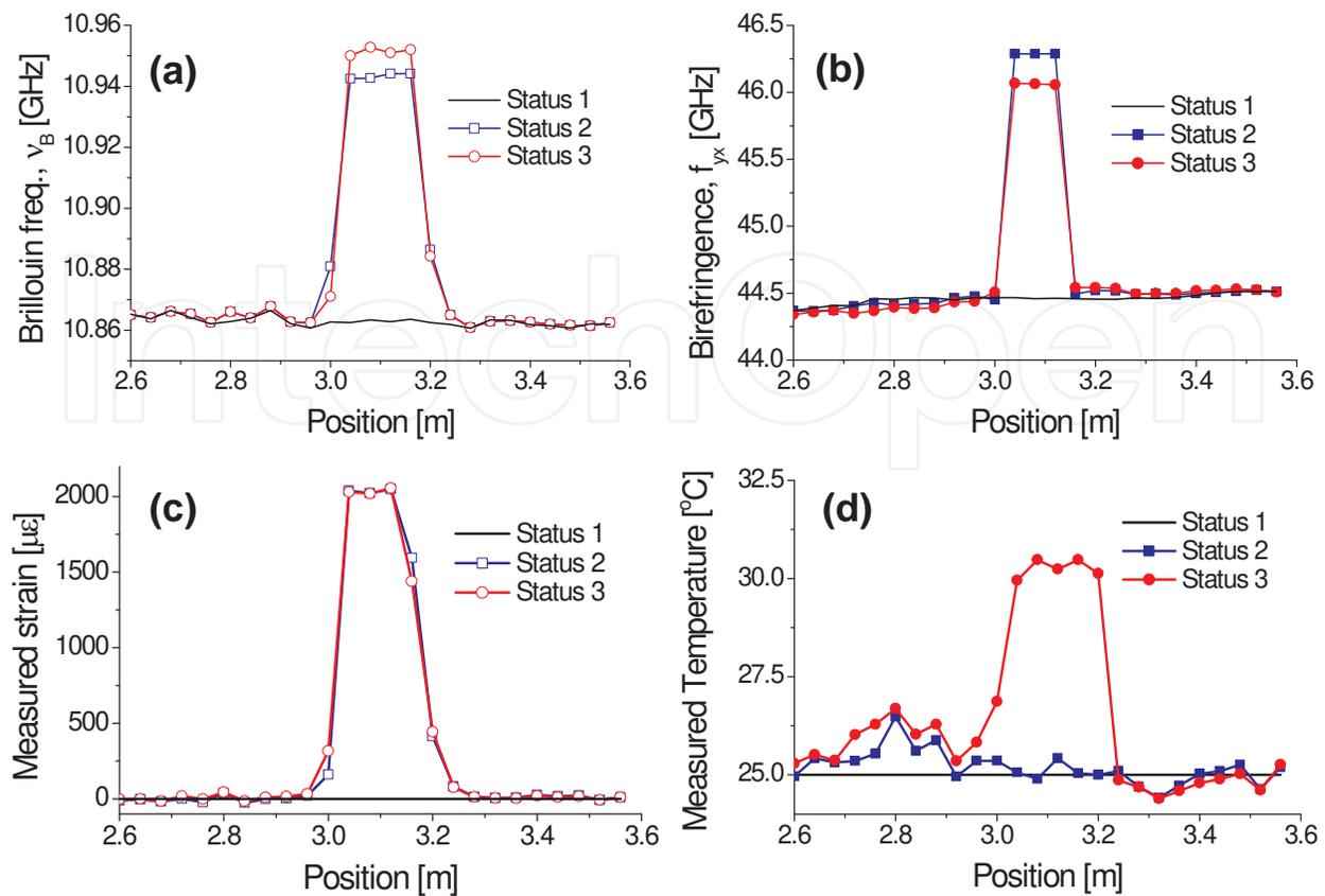
**Figure 23.** Experimental results of high-accuracy distributed discrimination of strain and temperature based on one-laser scheme. Distribution of Brillouin frequency shift (a), the birefringence-determined frequency deviation (b), strain (c), and temperature (d). (After Ref. [112]; © 2011 OSA.)
