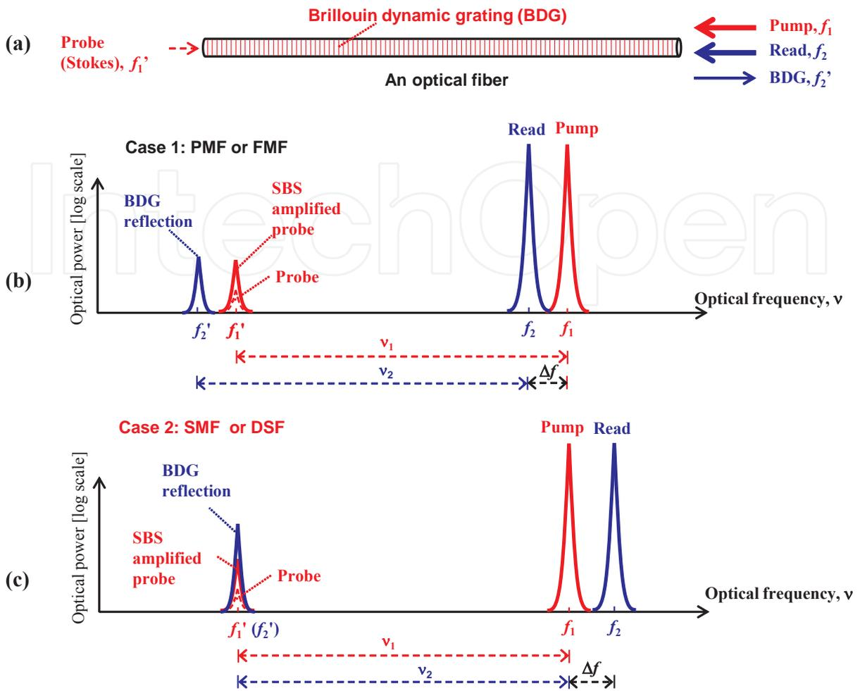
**Figure 13.** Principle of BDG in an optical fiber. (a): Orientation of optical injection. (b) and (c): Two different cases of the optical frequency relation among the pump, probe (Stokes), readout, and BDG reflection. (After Ref. [93]; © 2013 OSA.)
