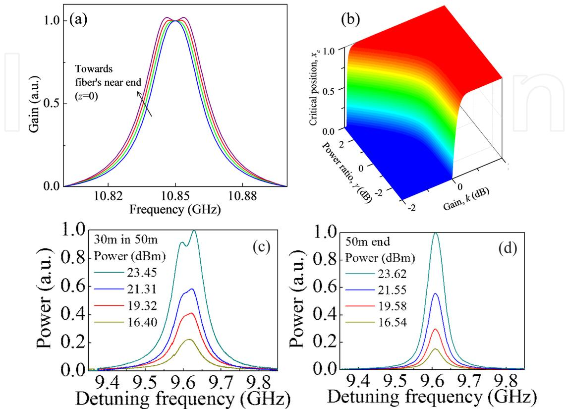
**Figure 8.** (a) Simulated BGS at different positions in the fiber. (b) Critical position  $x_c$  determined by the normalized gain  $k$  and injected power ratio  $\gamma$ . The critical positions divide the fiber into two parts with and without the spectral hole burning phenomenon. Measured BGS in the middle (c) or at the end (d) of a 50-m-long fiber. (after Ref. [42]; © 2014 JJAP.)
