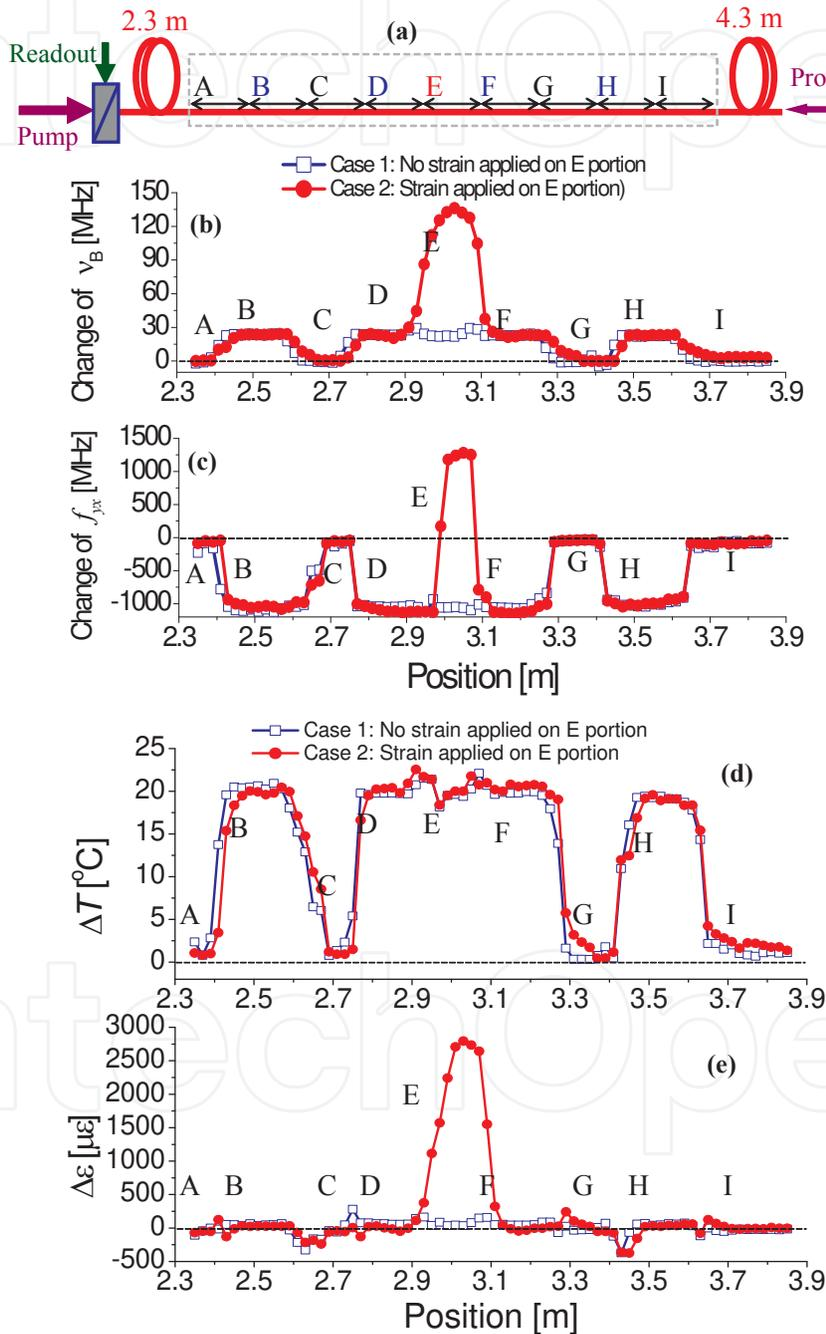
**Figure 20.** Preliminary experiment of distributed discrimination of strain and temperature based on two lasers modulated in frequency. (a) FUT configuration. Measured distribution of Brillouin frequency shift (b) and the birefringence-determined frequency deviation (c). Deduced distribution of temperature (d) and strain (e). (After Ref. [113]; © 2010 IEEE.)
