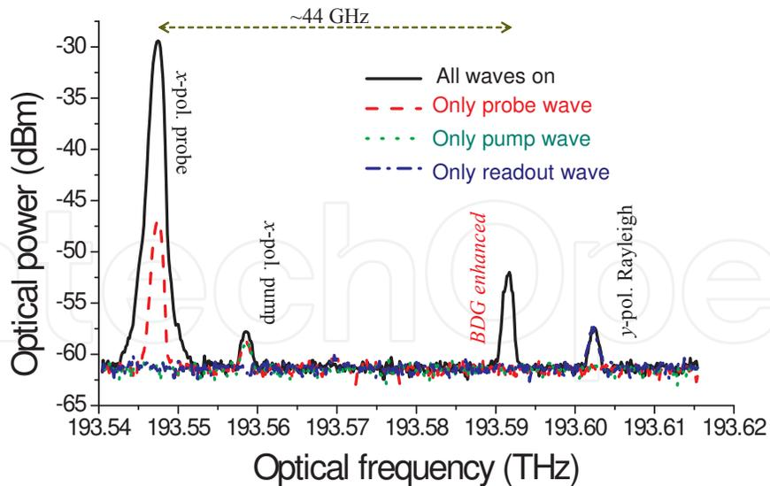
**Figure 14.** Qualitative characterization (optical spectra) of BDG reflection in a PMF with  $B=3.3 \times 10^{-4}$ . Black-solid, all pump, probe and readout waves are launched; blue-dash-dotted, only readout wave; red-dashed, only probe wave; green-dotted, only pump wave.
