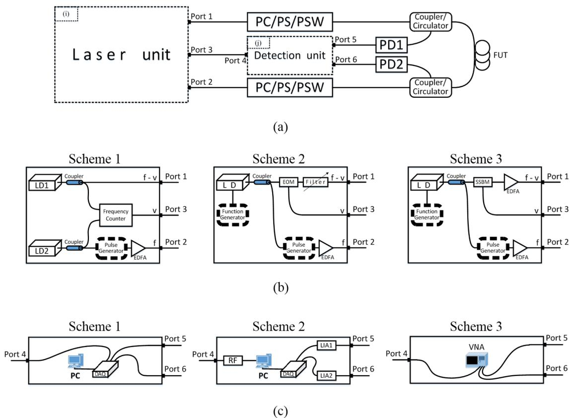
**Figure 6.** Experimental setup of BGS measurement based on stimulated Brillouin scattering (SBS). (a) Basic configuration. (b) Three different methods of laser unit (dotted box “i” in (a)) with two optical ports and one electrical port. The dashed boxes of Function Generator or Pulse generator are used for distributed SBS measurement. (c) Three schemes of detection unit shown in dotted box “j” in (a).
