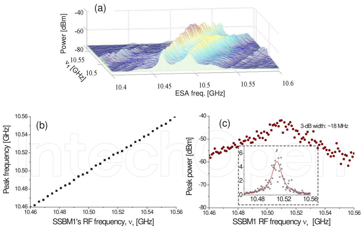
**Figure 15.** Characterization of the BDG reflection based on heterodyne detection. (a) 3D plot of electronic spectra of heterodyne detection when the pump-probe frequency offset ( $f_1-f_1'$ ) is scanned. Dependence of peak frequency (b) and power (c) of each spectrum on  $f_1-f_1'$ . The dashed inset denotes Lorentz fitting (solid curve) to the linear vertical scaled symbols in (c). (After Ref. [96]; © 2013 JJAP.)
