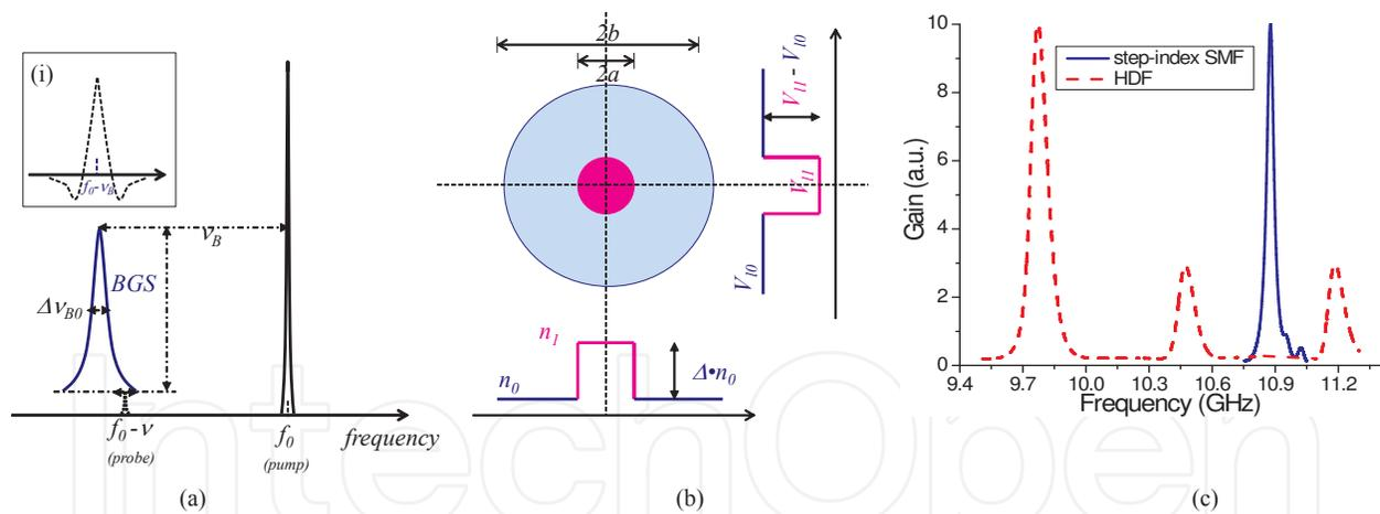
**Figure 3.** (a) Brillouin gain spectrum (BGS) in optical fibers. The inset “i” denotes the change of group velocity of optical fields. (b) Cross section of a step-index SMF.  $\Delta=(n_1-n_0)/n_0$  is the relative index difference between the core ( $n_1$ ) and the cladding ( $n_0$ ). (c) Measured BGS of a step-index SMF (solid curve) and of a 17.0-mol% high-delta fiber (dashed curve). (Fig. 3(c) after Ref. [13]; © 2008 OSA.)
