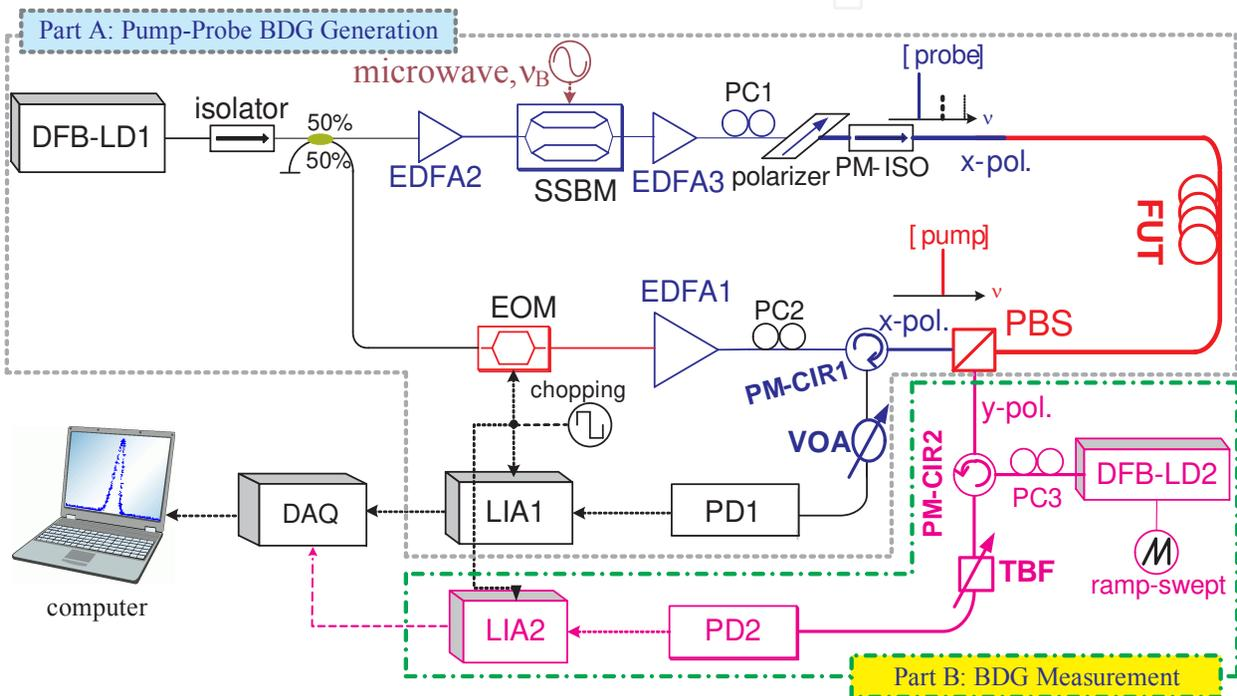
**Figure 16.** Configuration of the BDG characterization and strain-temperature discrimination. Part A, Pump-probe scheme to measure the BFS along  $x$ -axis and generate the BDG. Part B, Detection of the BDG diffraction spectrum to  $y$ -polarized readout wave. (After Ref. [89]; © 2009 OSA.)
