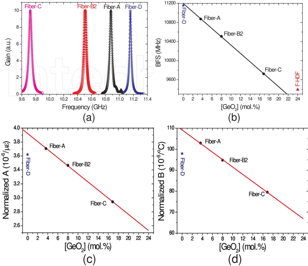
Figure 11. (a) BGS, (b) BFS, (c) normalized strain coefficient, and (d) normalized temperature coefficients in silica optical fibers with different GeO<sub>2</sub> concentration. (After Ref. [49]. © 2008 OSA/IEEE.)
