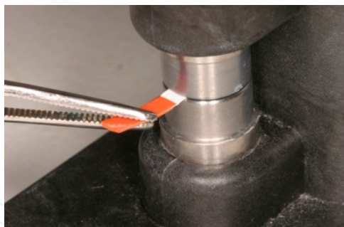
Figure 2. Crevicular fluid sample placement between Periotron® sensors.
