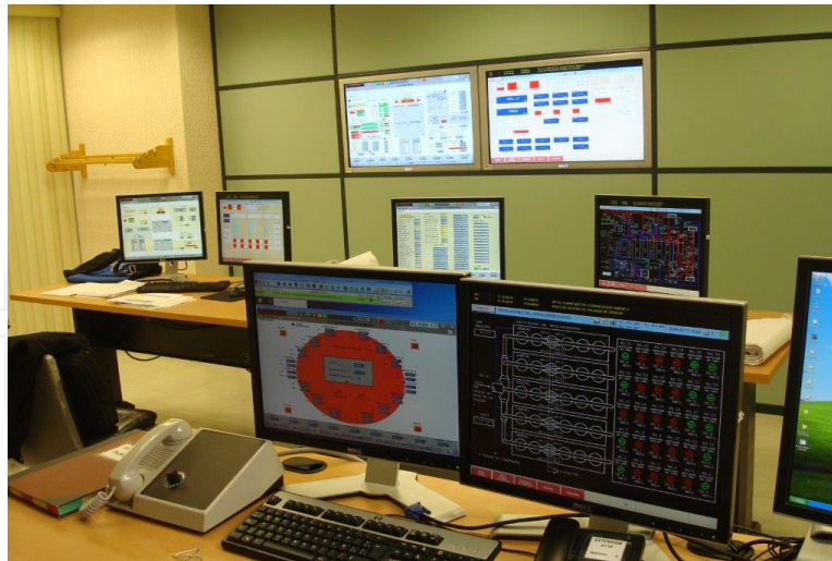
Figure 3. Hardware configuration (instructor and operation consoles)
