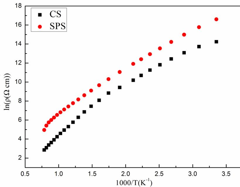
**Figure 9.** Temperature dependence of electrical resistivity  $\rho$  of the samples  $0.4\text{MgAl}_2\text{O}_4-0.6\text{YCr}_{0.5}\text{Mn}_{0.5}\text{O}_3$  sintered by conventional sintering (CS) and SPS [12].
