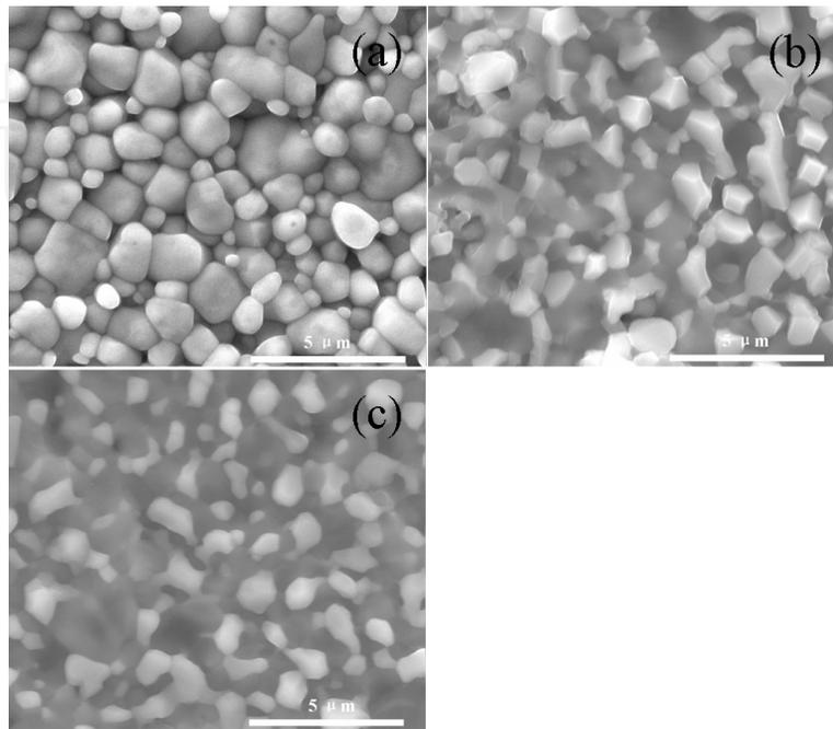
**Figure 8.** SEM images of the SPS-sintered  $x\text{MgAl}_2\text{O}_4-(1-x)\text{YCr}_{0.5}\text{Mn}_{0.5}\text{O}_3$  composite ceramics: (a)  $x=0.1$ ; (b)  $x=0.4$ ; (c)  $x=0.6$  [12].
