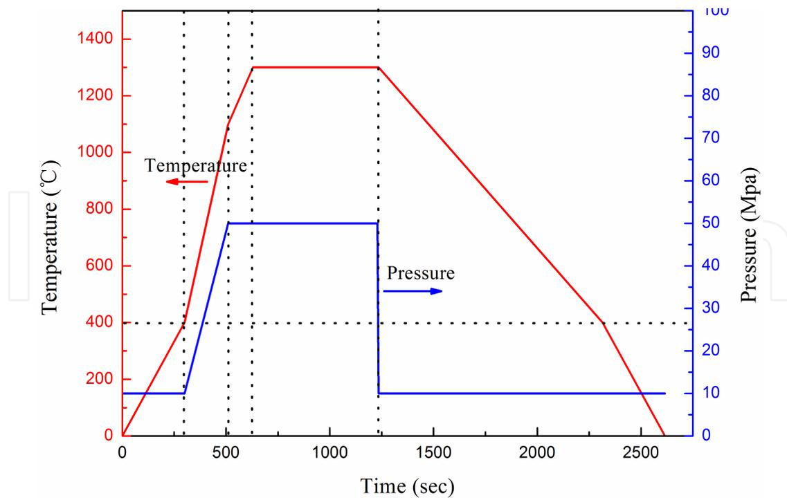
Figure 4. Time dependence of the temperature and applied pressure during SPS process [33].
