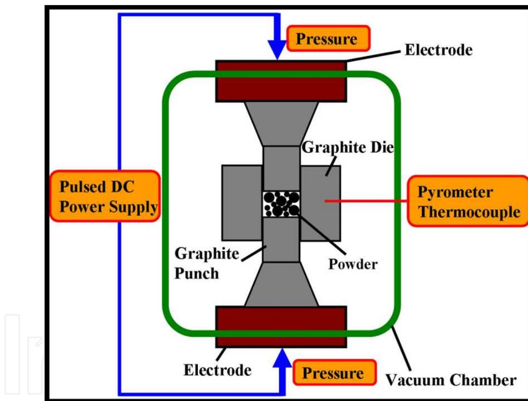
Figure 1. Schematic of SPS furnace [16].
