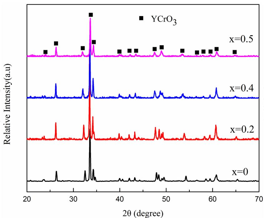
Figure 5. XRD patterns of the SPS-sintered  $\text{YCr}_{1-x}\text{Mn}_x\text{O}_3$  ceramics [32].
