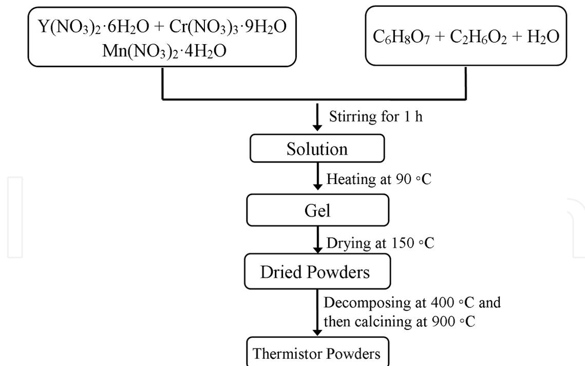
**Figure 2.** Flow chart for the fabrication of  $\text{YCr}_{1-x}\text{Mn}_x\text{O}_3$  thermistor powders by a Pechini method.
