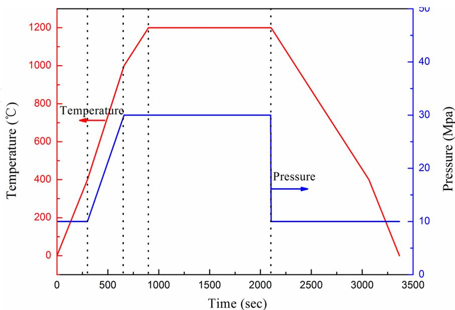
**Figure 7.** Time dependence of the temperature and applied pressure during SPS process.
