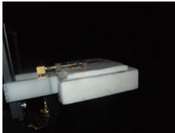
Figure 33. Antenna on the skin-equivalent phantom.
