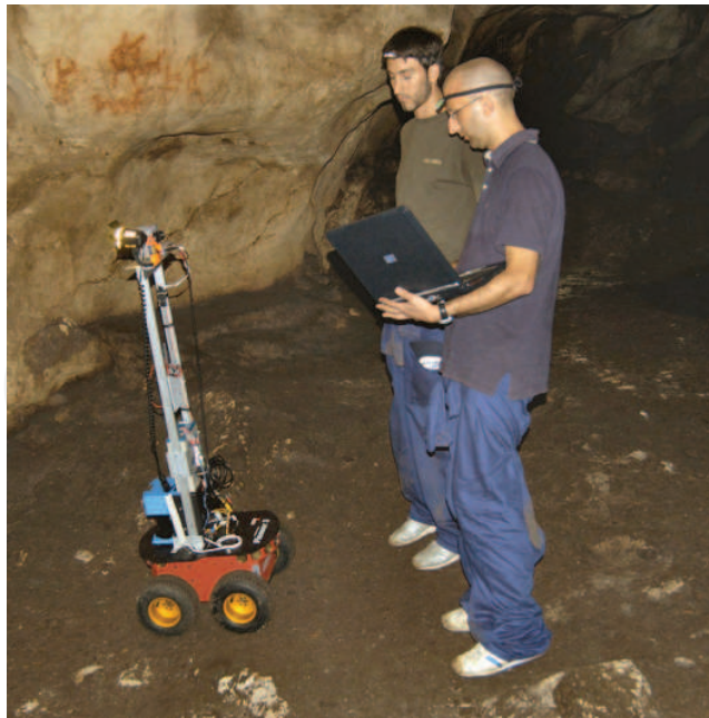
Fig. 2. The mobile robotic platform in the configuration used in the cave.
