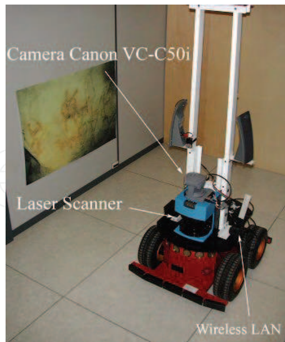
Fig. 1. The robotic mobile platform in the configuration used in the polygonal environment.
