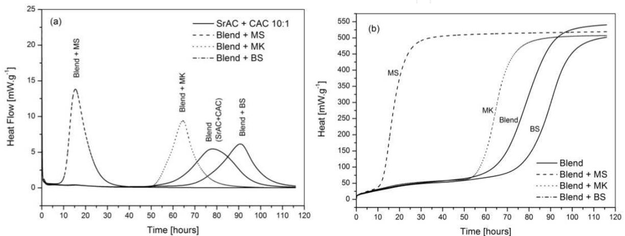
**Figure 13.** Heat flow (a) and heat of hydration (b) released from the multicomponent cement during the first 128 h of hydration from the blend of CAC and SrC (1:10) with microsilica (MS), metakaolinite (MK) and blast furnace slag (BS).
