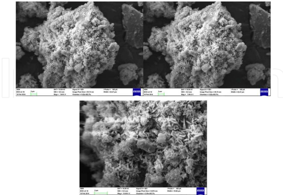
Figure 11. The hydrated cement stone prepared from the mixture of SrAC and PC (1:3).
