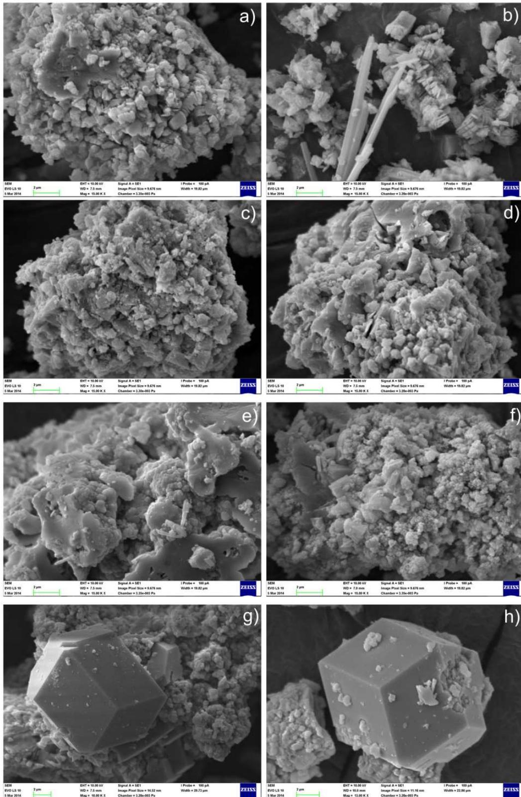
**Figure 29.** Electron microscopy of hydrated cement stone of clinker prepared with 5 % of  $B_2O_3$ (a),  $Fe_2O_3$  (b)  $Y_2O_3$ (c),  $V_2O_5$  (d),  $ZrO_2$  (e),  $MnO$  (f) and  $ZnO$  (g) with well developed crystal of  $Sr_3AH_6$  (h).
