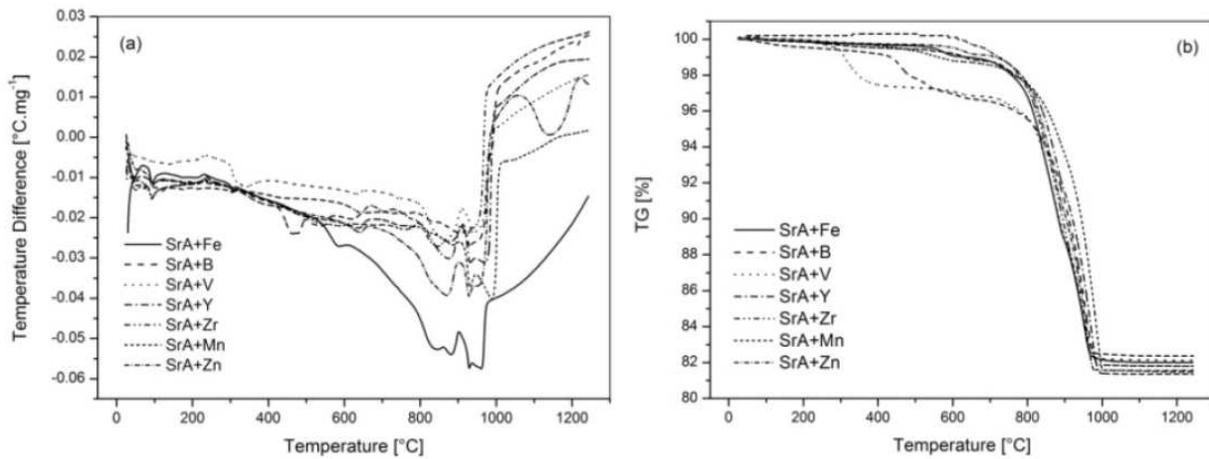
Figure 26. Thermal analysis of raw meals heated at the rate of 10 °C min<sup>-1</sup>: DTA (a) and TG (b).
