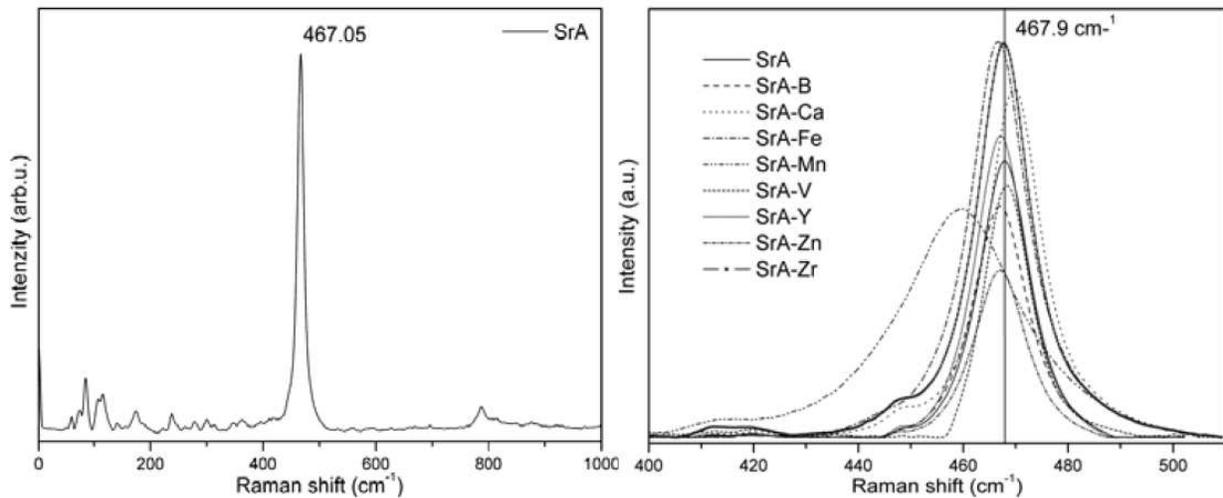
**Figure 30.** Raman spectra of  $\text{SrAl}_2\text{O}_4$  phase (a) and doped  $\text{SrAlO}_4$  structures (b) (where =Ca, Zn, Mn and =B, Fe, V, Y, Zr in substitution of 5 wt.%).
