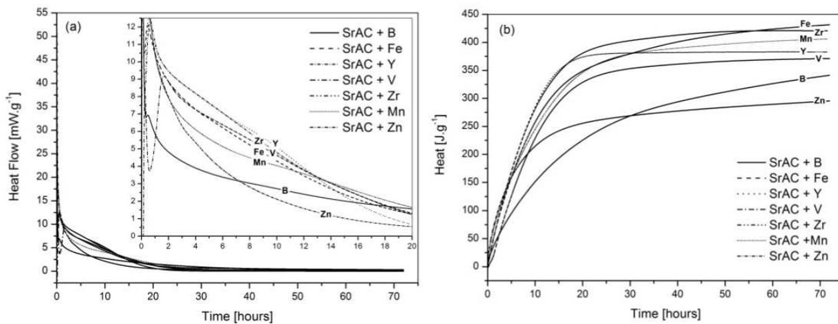
Figure 28. Hydration of clinker prepared with dopants.
